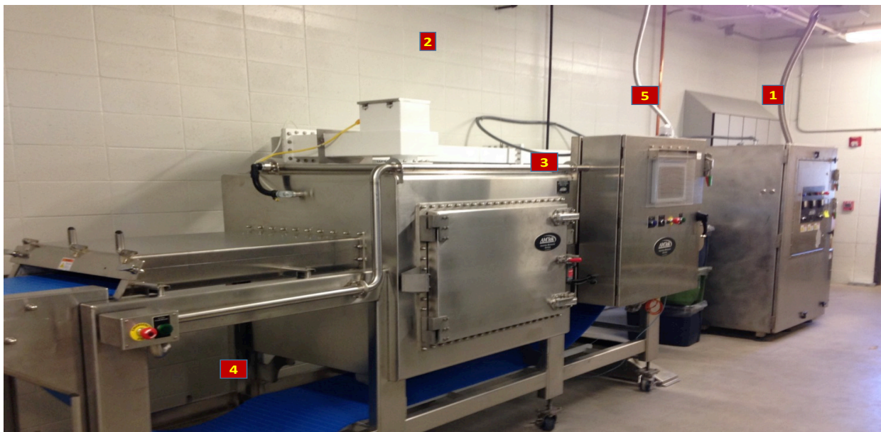
Figure 2.1: Industrial type microwave used in the showing the transmitter (1), wave guide (2), heating zone (3), the conveyor belt (4), and control panel (5).
