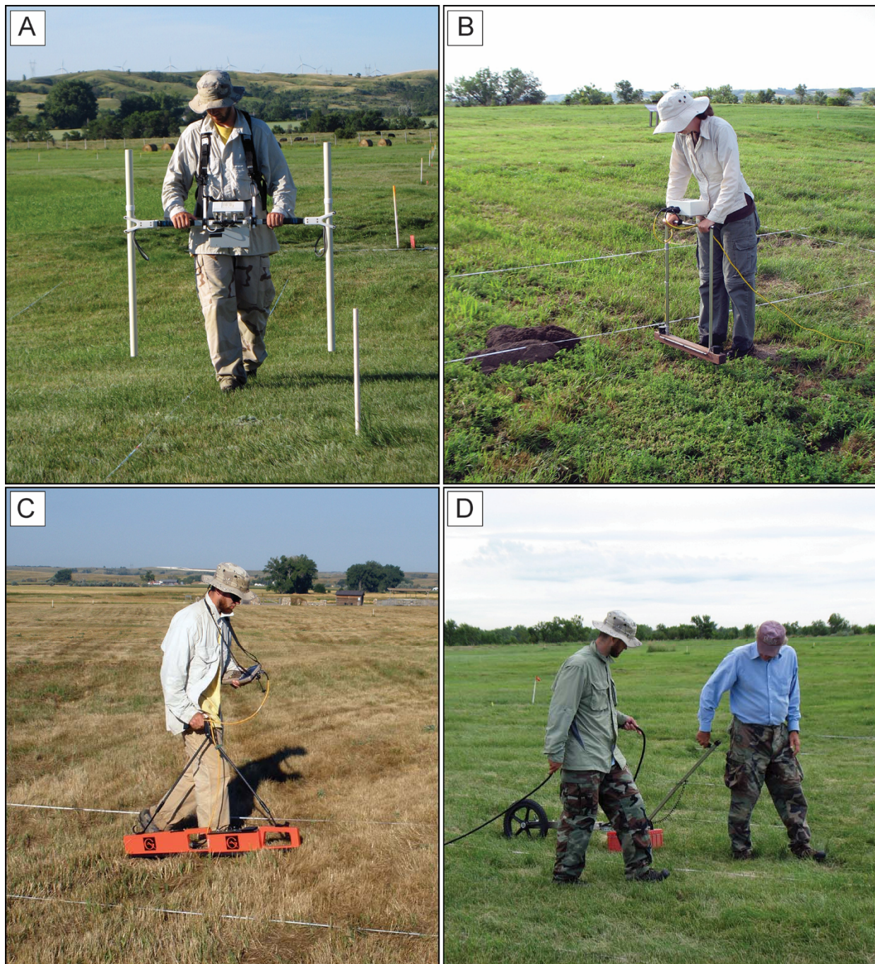
Figure 2.1. Geophysical instruments employed in surveys: a) Bartington Grad601 dual fluxgate magnetic gradiometer; b) TR Systems Ltd. TR/CIA resistivity meter (Geoscan Research RM-15 resistance meter not shown); c) Geonics Ltd. EM38B electromagnetic induction meter; and d) Geophysical Survey Systems, Inc., SIR-2000 ground-penetrating radar. Photographs by the author.
