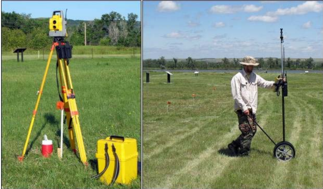
Figure 2.2. The Trimble 5600 robotic total station (left) and wheeled reflector rod (right). A data logger and digital display mounted to the reflector rod allows the instrument operator to view his or her location in real time. Photographs by the author.
