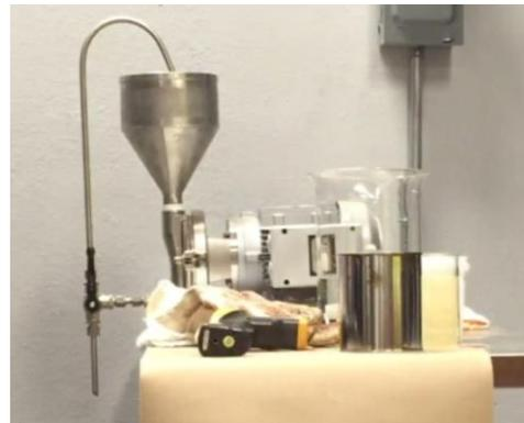
**Figure 6. University of Arkansas Raschig Mill**
