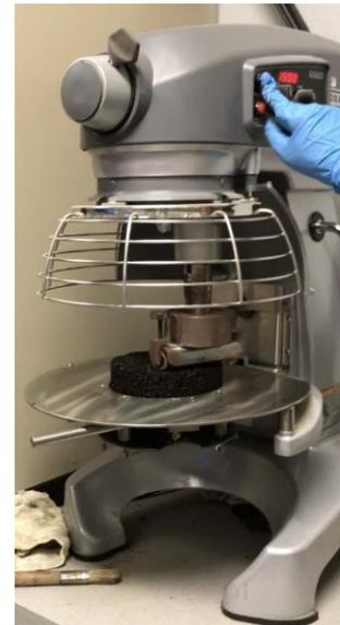
**Figure 16. Hobart mixer for raveling test**
