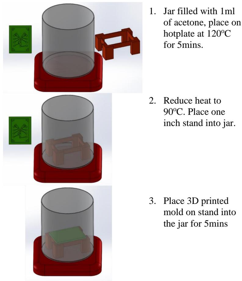
Figure 2.22: Process flow of Acetone vapor bath procedure
