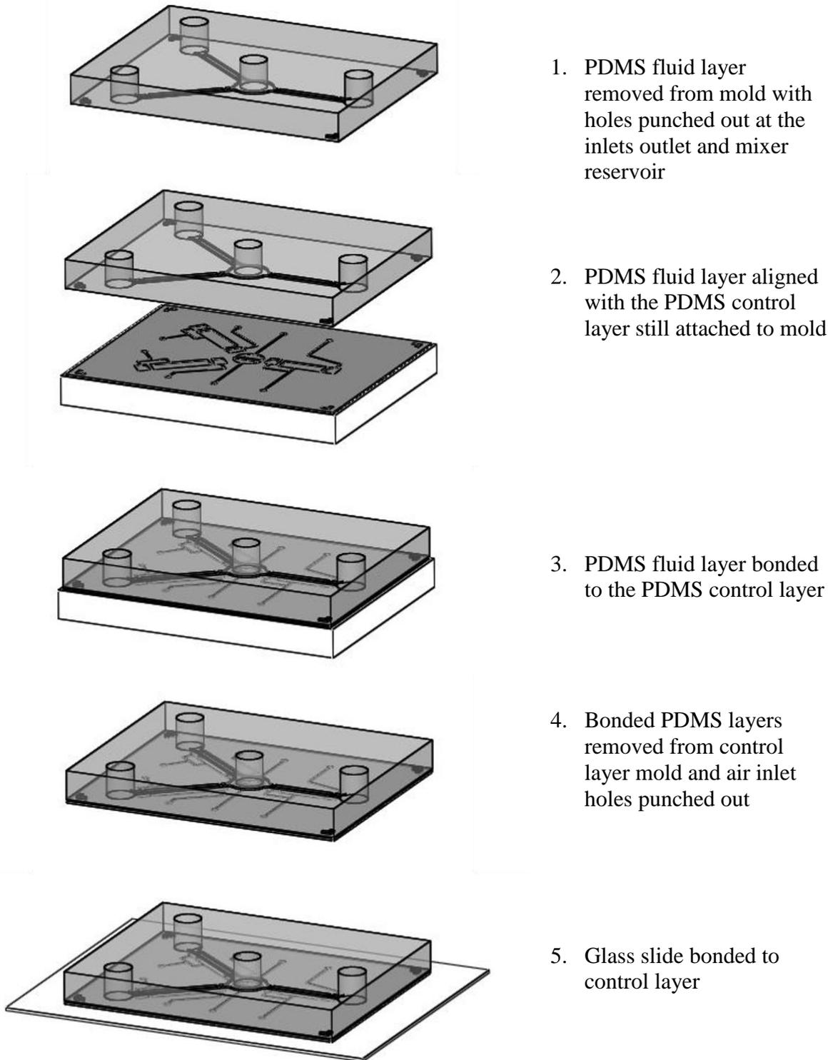
Figure 2.15 Process flow for bonding and assembling PDMS device
