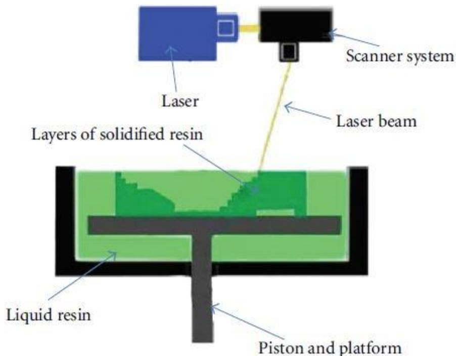
Figure 1.4: Diagram of Stereo-lithography 3D Printing [20]
