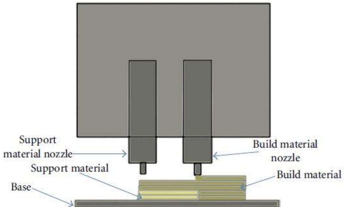
Figure 1.5: Diagram of Fused Deposition Modeling 3D Printing [21]
