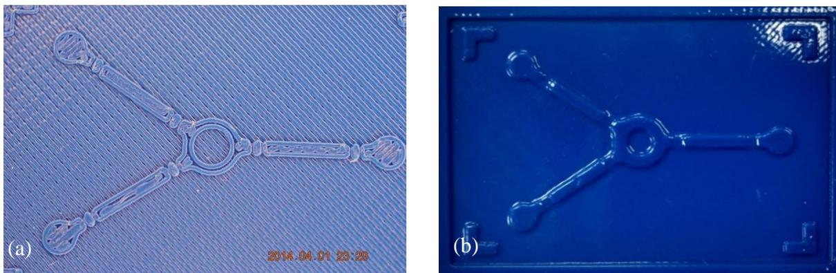
Figure 2.23: Image (a): 3D printed master mold of fluid layer before AVB surface treatment
