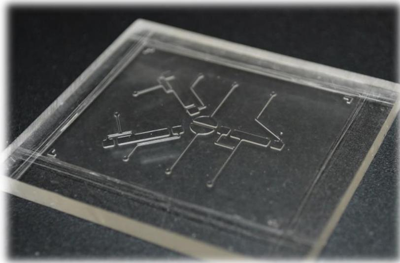
Figure 2.8: Micro-engraved PMMA master mold of control layer
