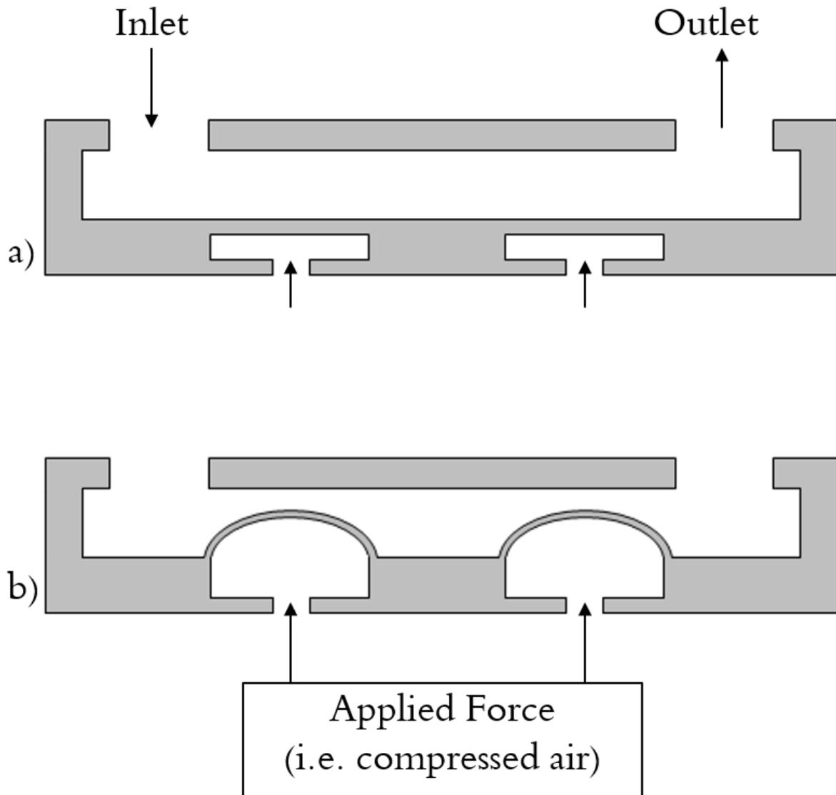
Figure 1.2: Mechanical micro-pump with actuating diaphragms. Image (a): Diaphragms at rest
