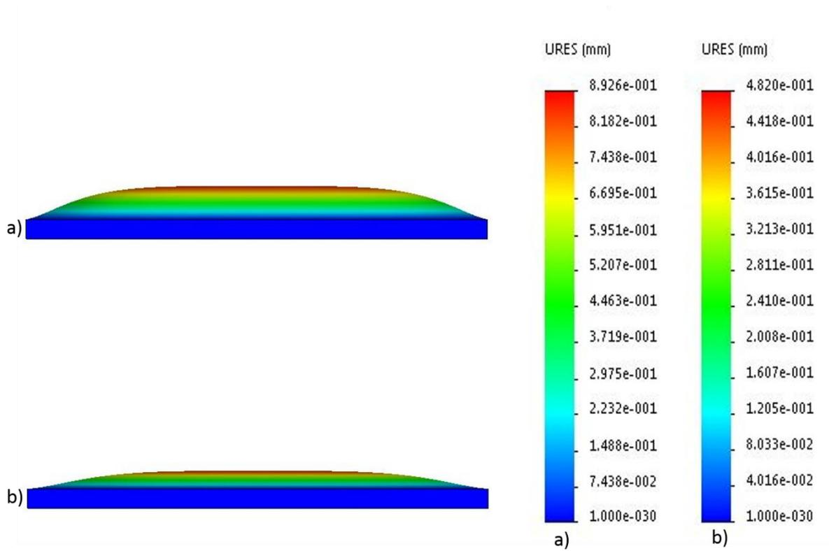
Figure 3.12: SolidWorks Diaphragm Deflection Simulation. Image (a): Maximum Deflection
