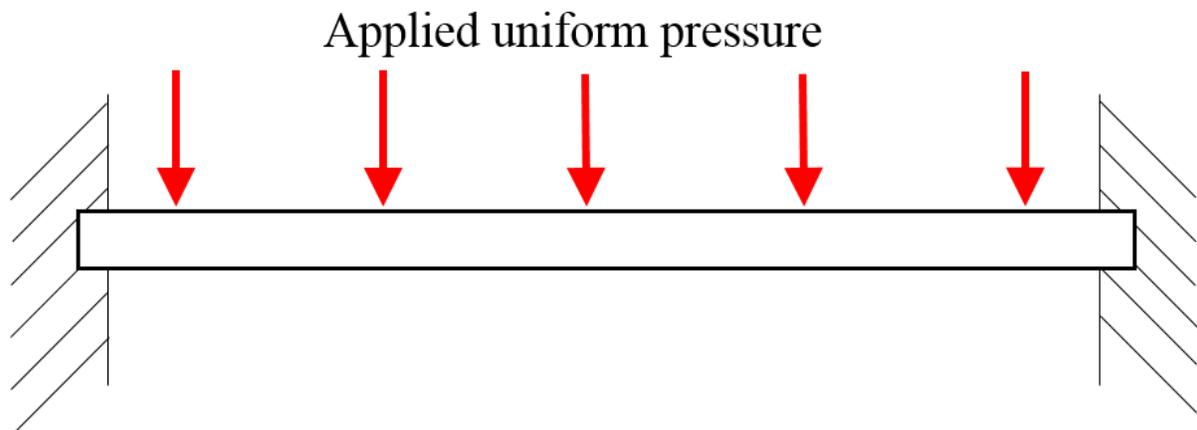
Figure 3.13: Flat plate with clamped edges and applied uniform pressure
