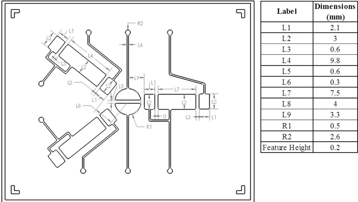
Figure 2.5: PMMA mold design of control layer
