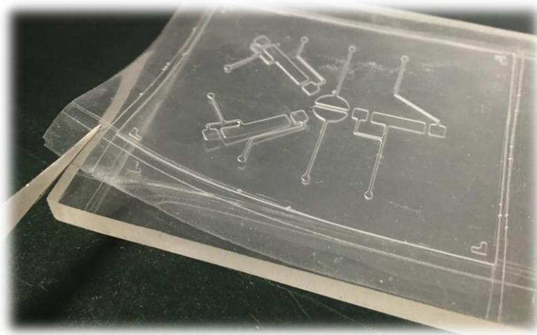
Figure 2.13: Casted PDMS control layer and mold
