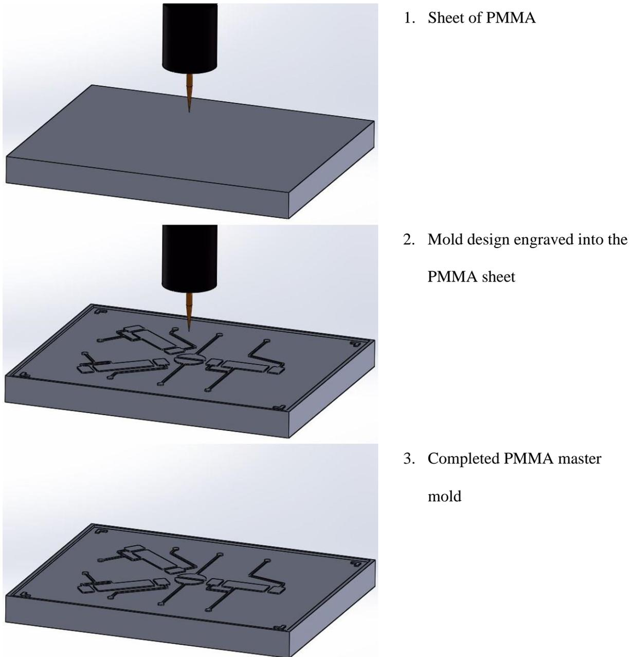
Figure 2.7: Micro-engraving process flow of master mold
