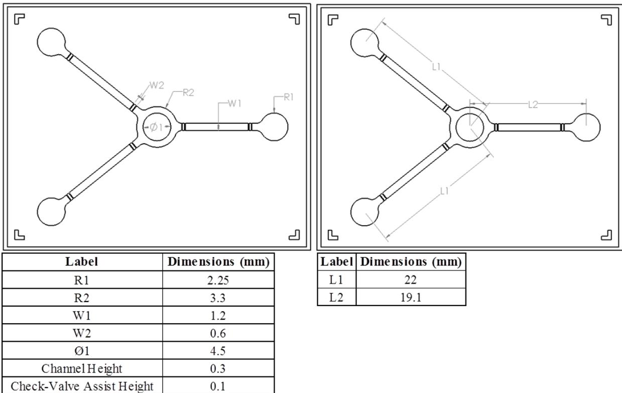
Figure 2.4: PMMA mold design of fluidic layer micro-channel
