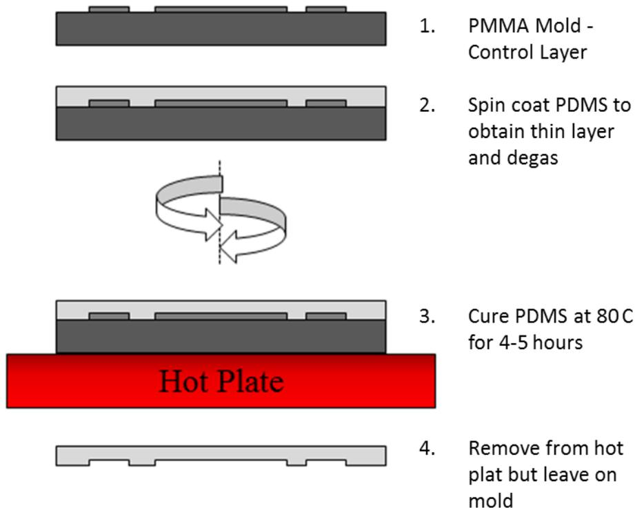
Figure 2.11: Control layer casting process
