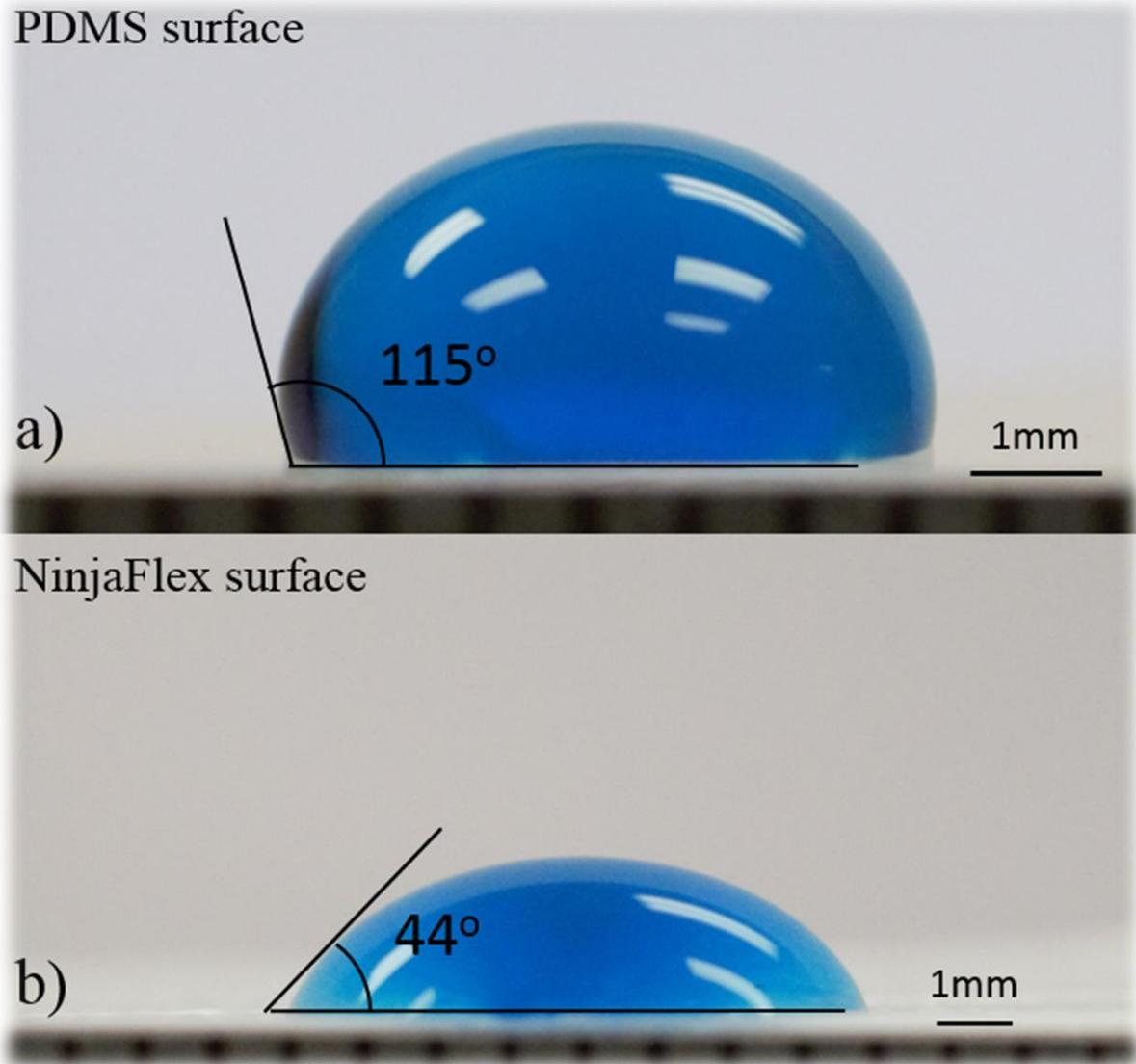
Figure 2.39: Image (a): Hydrophobic test of PDMS with contact angle of about  $115^\circ$
