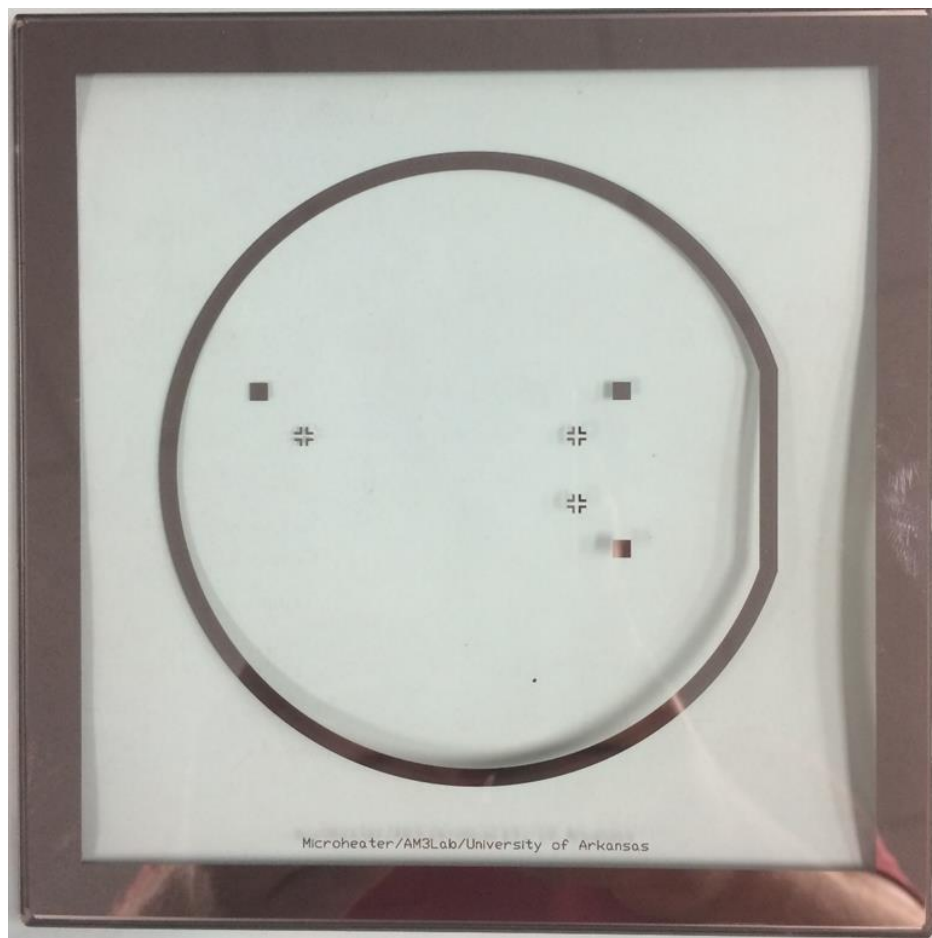
Figure 25- Digital Design of PhotoMask for Microheater Arrays
