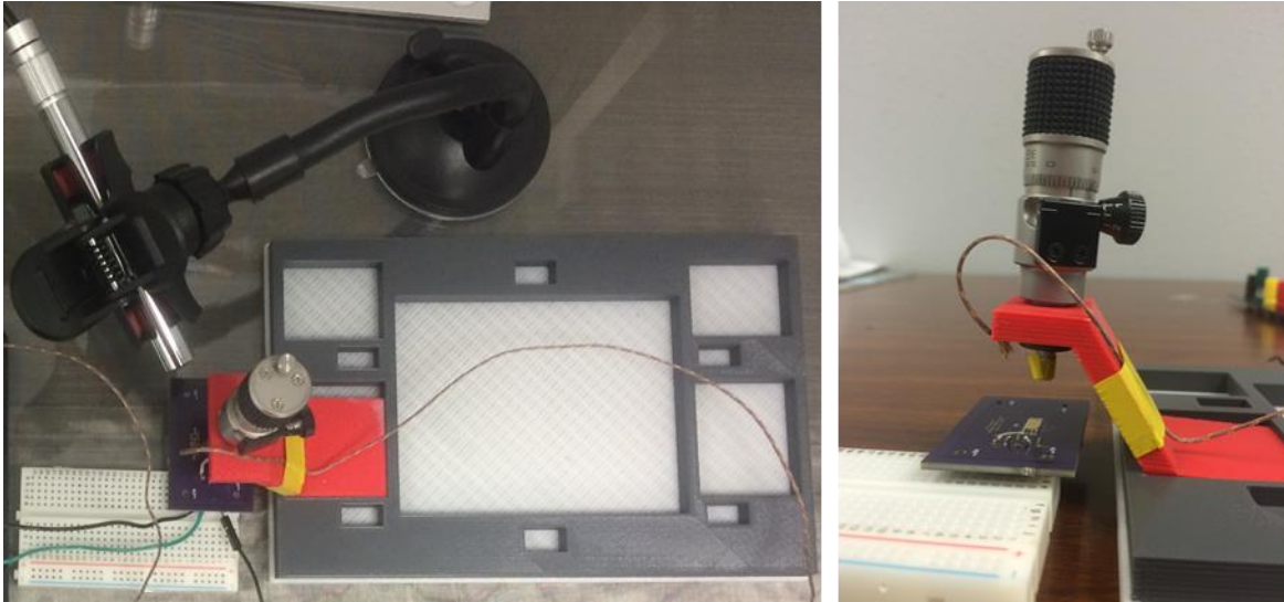
Figure 38-Thermocouple and Camera Setup for Test 3
