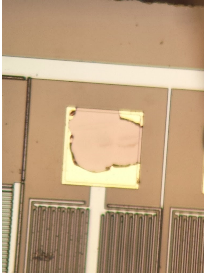
Fig. 6.1. Bonding pad from the first pass after attempting 1 mil gold ball bonding three times. The gold coating on the pad (yellow) has been torn off where the ball bonds were made, leaving the underlying metal below.
