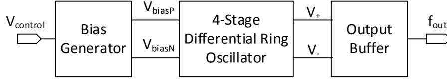
Fig. 6.6. Updated block diagram of the tapeout 2 VCO.
