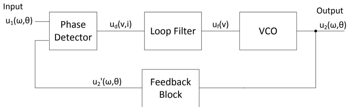
**Fig. 2.6. General control-loop topology of a PLL.**
