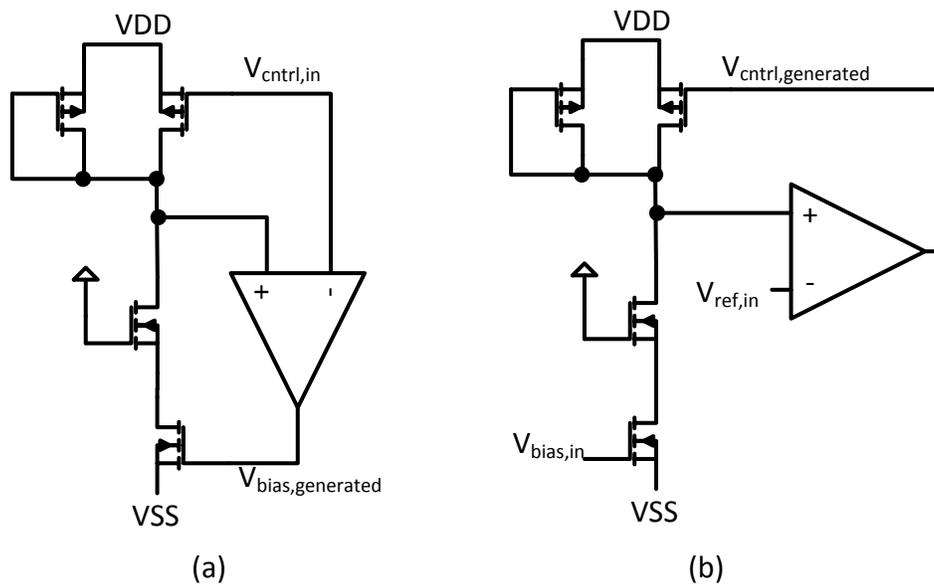
**Fig. 2.17. Half-buffer replica biasing circuits for the Maneatis delay cell. The circuit in (a) has a single control input voltage that sets the bias current and the delay cell output swing, while the circuit in (b) forces the output swing to be fixed at  $V_{ref}$ , and  $V_{bias,in}$  is provided to the delay cells as well.**
