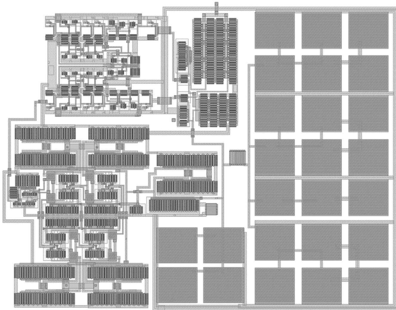
**Fig. 6.19. Complete PLL for Tapeout 2. The PFD is on the top left, the Charge Pump is rotated 90° and is in the top middle. The primary loop capacitor is on the right and the VCO is on the lower left.**
