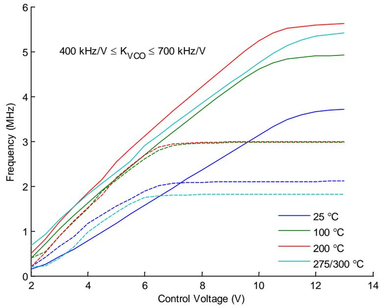
**Fig. 5.8. Simulation of the VCO with models before Tapeout 1 (solid lines) and models derived from test devices returned on Tapeout 1 (dashed lines). Although the gain is similar in the controllable region, the large shift in the PFET threshold voltage limits the VCO to an operating frequency of 2-3 MHz.**
