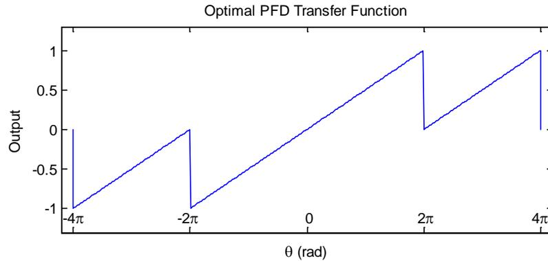
**Fig. 4.4. Optimal transfer function for a phase-frequency detector.**
