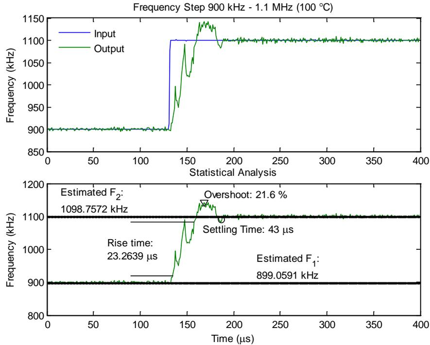
**Fig. 5.18. Step Response of the PLL at 100 °C.**
