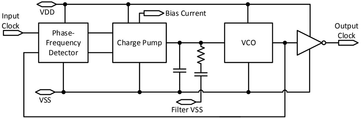
**Fig. 4.18. Final system diagram used for layout.**
