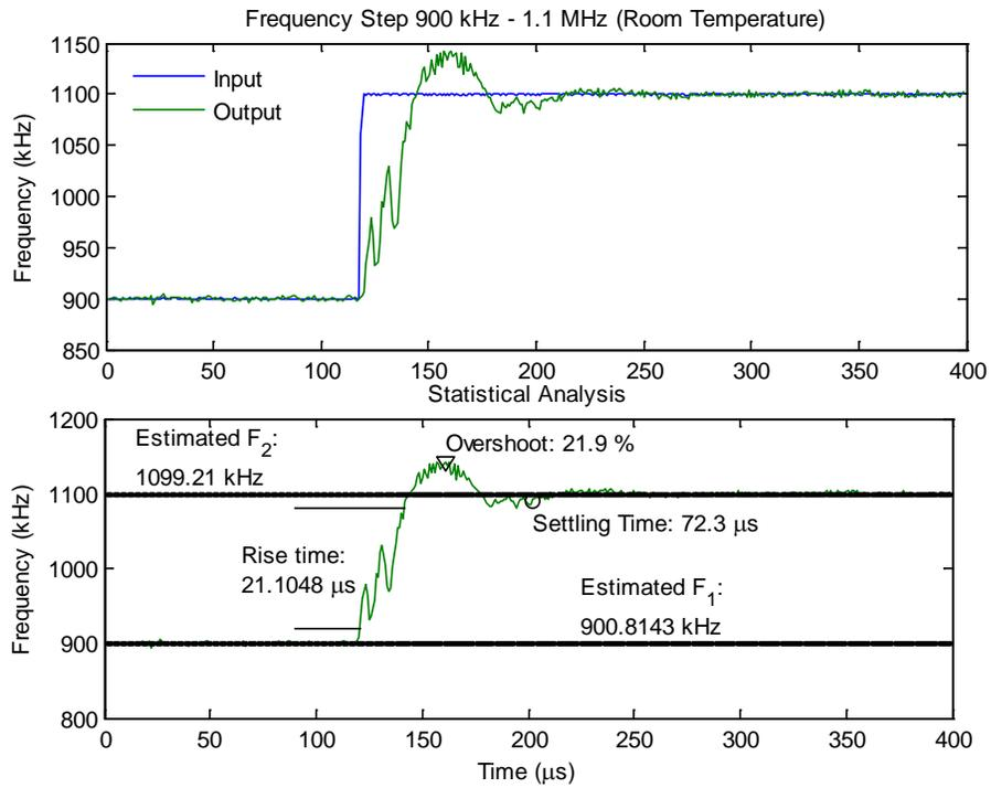
**Fig. 5.17. Step Response of the PLL at room-temperature.**
