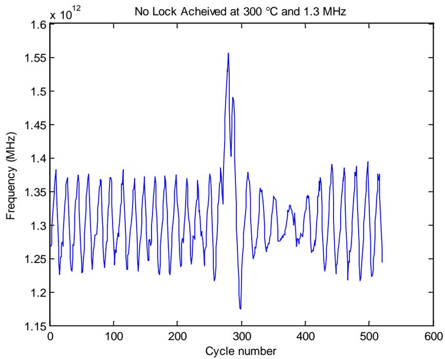
**Fig. 5.15. Failure to lock at 300 °C.**
