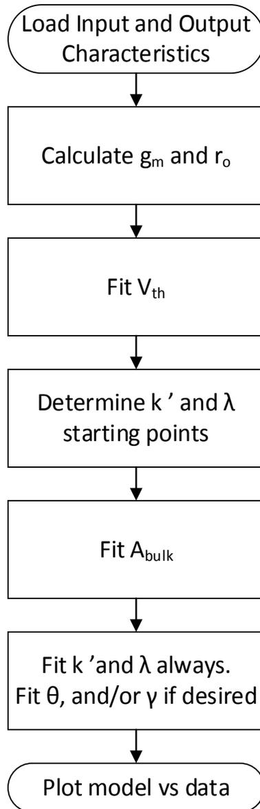
**Fig. 3.13 Simplified flowchart of the fitting algorithm.**
