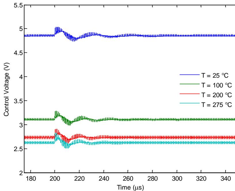
**Fig. 4.20. Control voltages during the +90° input phase step.**
