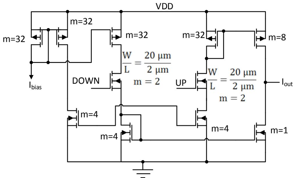
**Fig. 6.4. Updated charge pump schematic for tapeout 2.**
