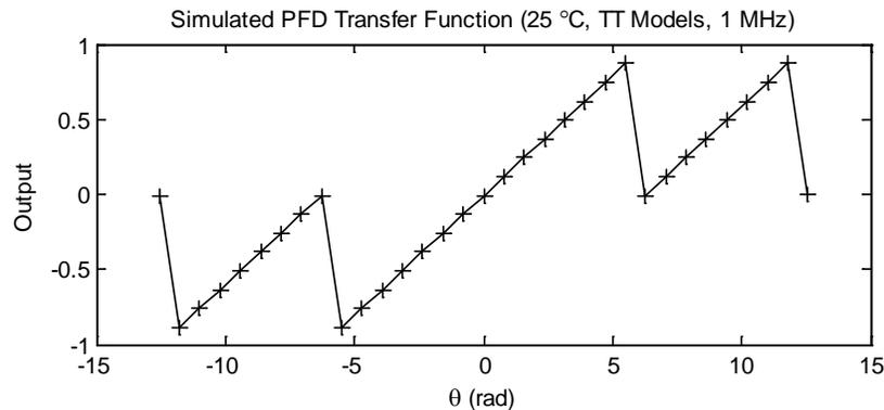
**Fig. 4.5. Simulated transfer function of the standard PFD.**
