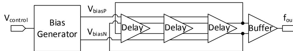
**Fig. 4.14. Block-level diagram of the Voltage Controlled Oscillator.**
