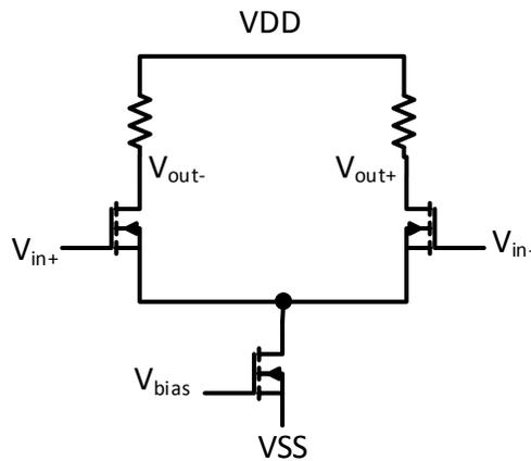
**Fig. 2.14. Differential delay cell with resistive loads.**
