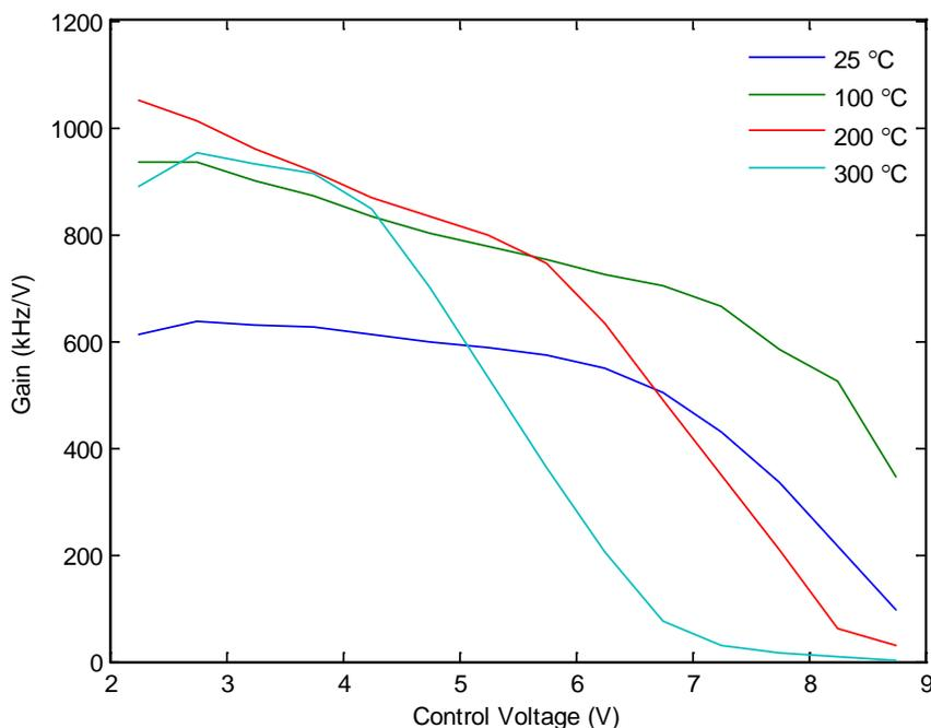
**Fig. 6.10. VCO gain vs control voltage for tapeout 2.**
