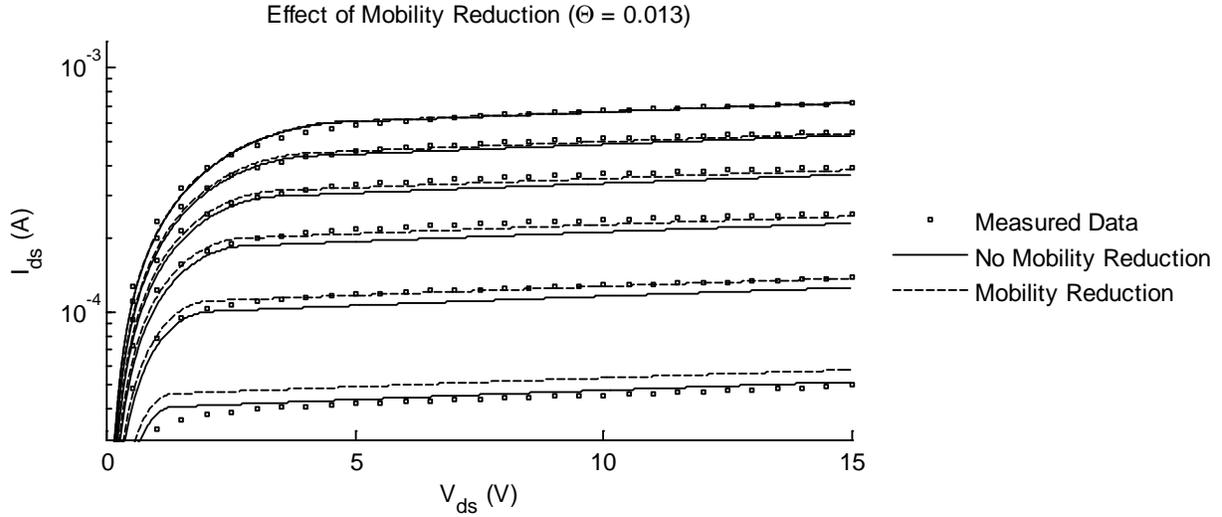
**Fig. 3.10.** Effect of mobility reduction on curve fitting for N-FETs for tapeout 2 with  $v_{gs}=5, 7, 9, 11, 13,$  and  $15$  V. Some improvement in fitting is visible from  $7$  V and up, but at  $5$  V, the fit without mobility reduction is better.
