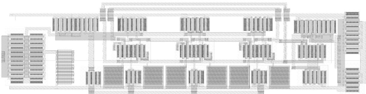
**Fig. 4.25. Layout of the VCO. VDD runs along the top and VSS runs along the bottom. The current-mirror load delay cells are in the center. The bias generator and  $V_{\text{control}}$  input are on the left. The output buffer is on the right.**
