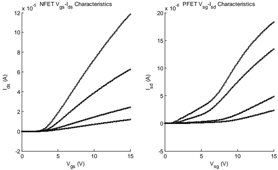
**Fig. 2.3. NFET and PFET characteristics at  $V_{gs}$  ( $V_{sg}$ ) = 5 V at room temperature.  $W/L = 20 \mu\text{m}/1.2 \mu\text{m}$ ,  $20 \mu\text{m}/2 \mu\text{m}$ ,  $20 \mu\text{m}/5 \mu\text{m}$ , and  $20 \mu\text{m}/10 \mu\text{m}$ .**
