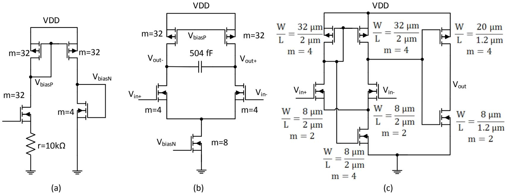
Fig. 6.7. Updated Block Schematics for the VCO for tapeout 2. (a) Bias generator (b) Differential delay stage, and (c) output buffer.
