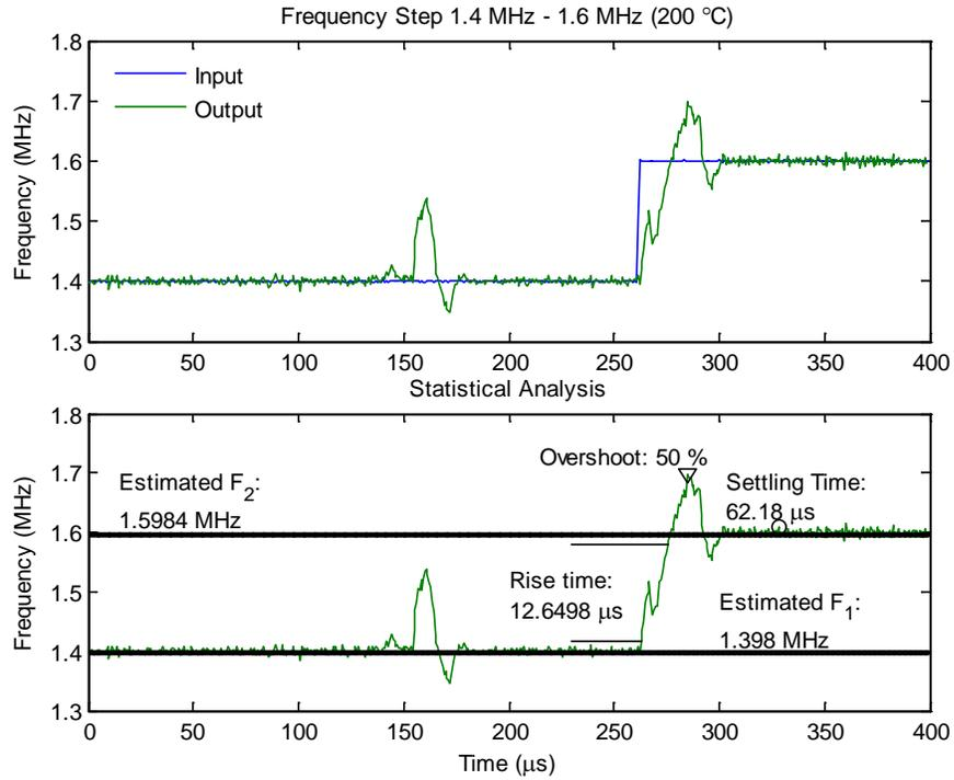
**Fig. 5.19. Step Response of the PLL at 200 °C.**
