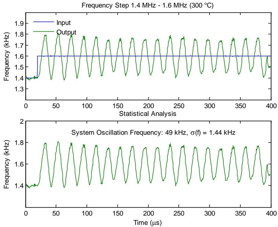
**Fig. 5.20. Step Response of the PLL at 300 °C.**
