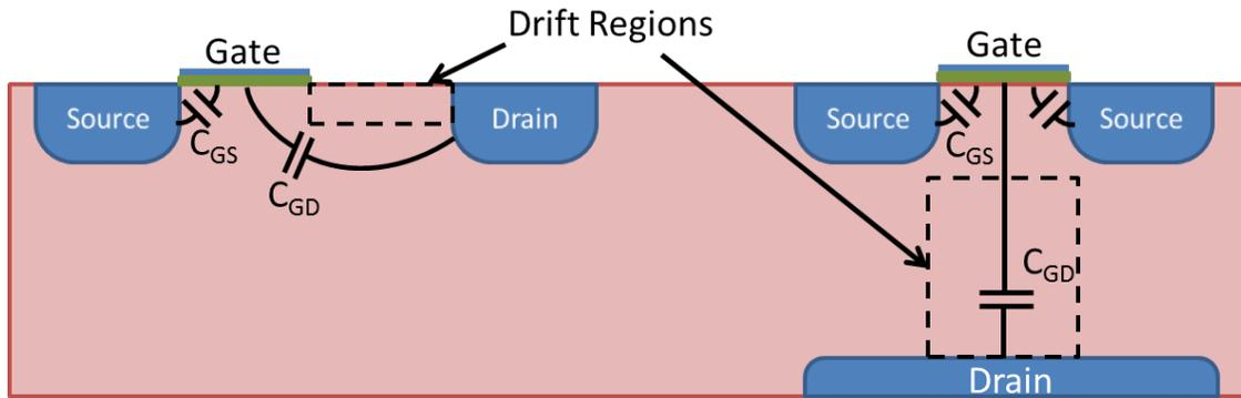
**Fig. 2.1. Drift Regions in Lateral and Vertical MOSFETs.**
