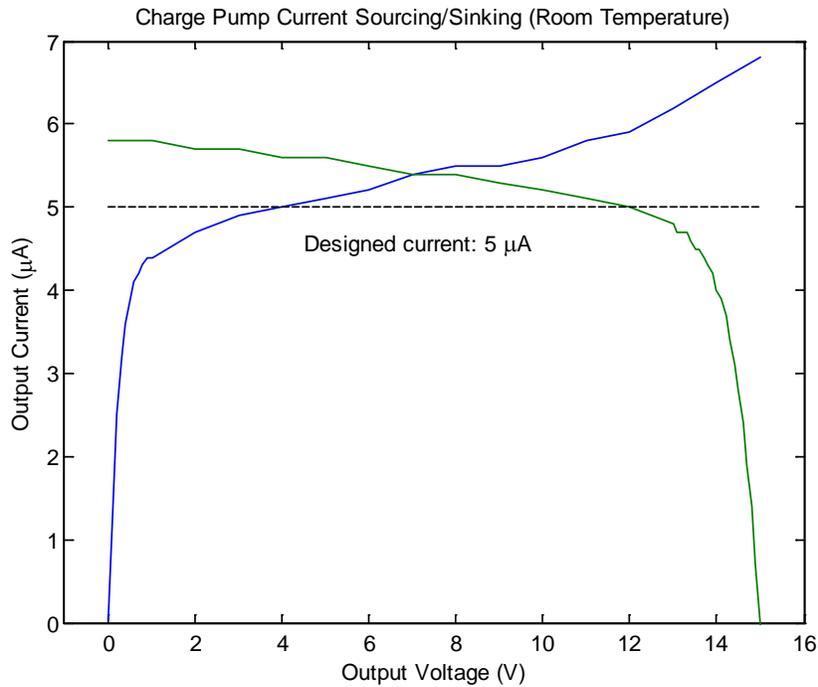
**Fig. 5.3. Current drive from the charge pump at DC and room temperature. Blue is the current-sinking mode, and green is the current-sourcing mode.**
