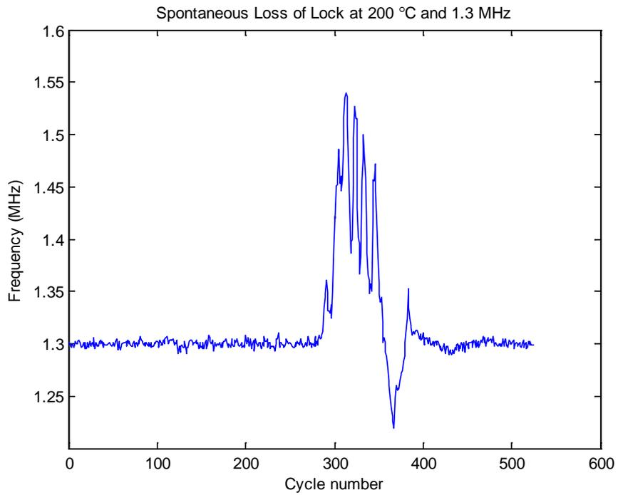
**Fig. 5.13. Spontaneous loss of lock at 200 °C.**
