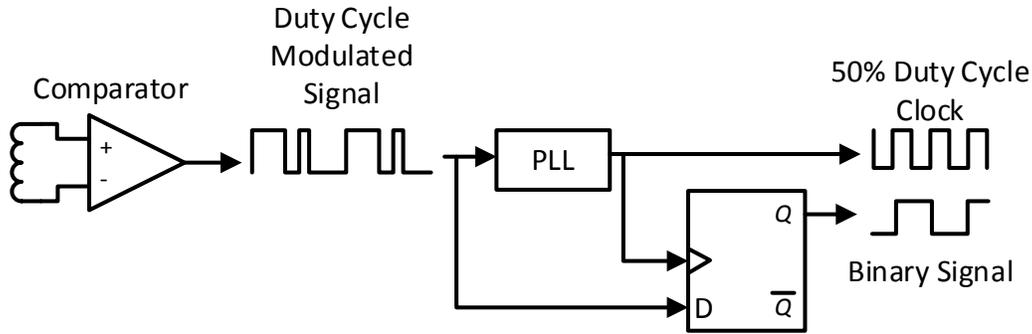
**Fig. 1.2. An isolated data transmission system utilizing the described PLL along with a comparator and D flip-flop.**
