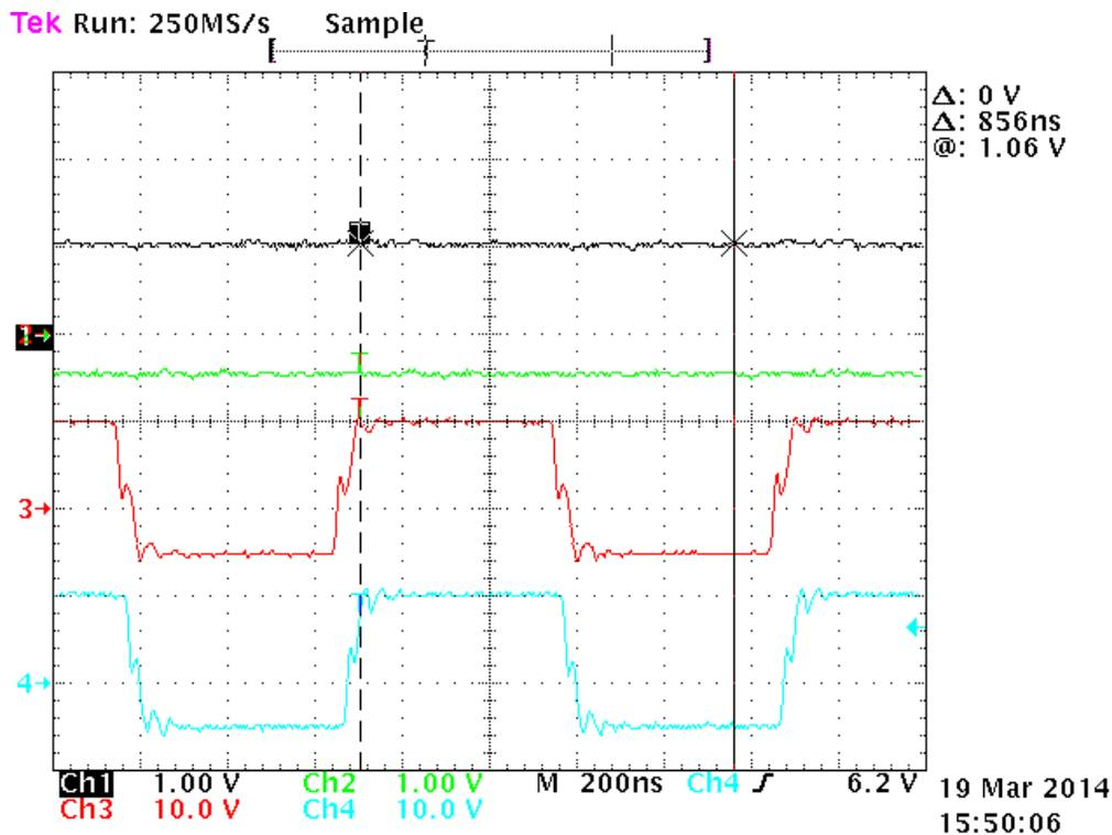
**Fig. 5.5. Transient testing of the PFD at 1 MHz. Channel assignments are the same as the previous figure. In this case, the DCLK input very slightly leads the CLK input, and neither output is asserted.**
