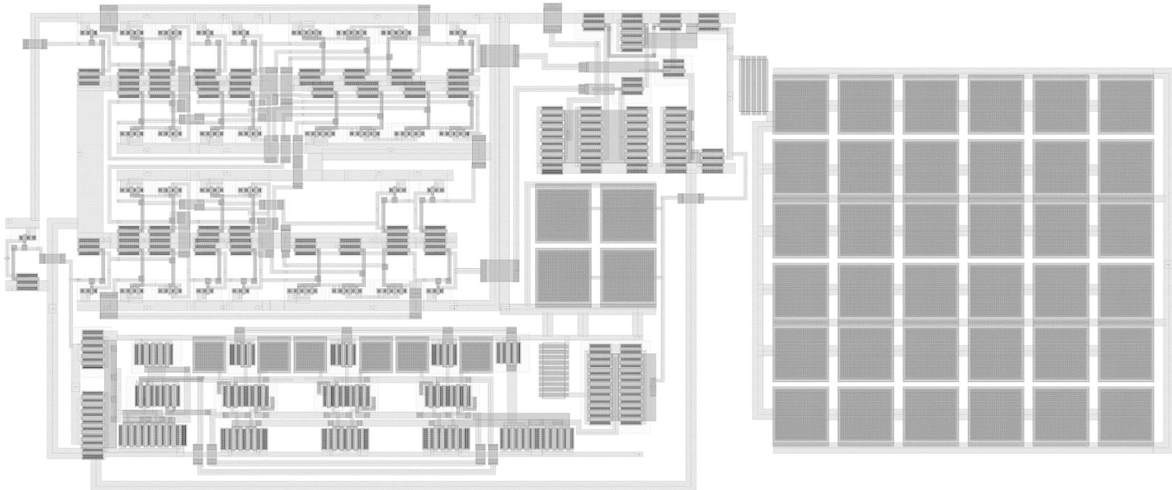
**Fig. 4.26. Complete PLL layout. The PFD is on the top left, the charge pump is at top center, and the VCO, rotated 180°, is in the lower left. On the right is the 54 pF capacitor broken into 36 1.5 pF tiled capacitors. The secondary capacitor, consisting of 4 1.5 pF tiled capacitors, is seen in the middle.**
