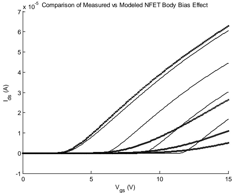
**Fig. 2.5. Comparison of measured and modeled body bias effects in the NFET with  $W/L = 20 \mu\text{m}/2 \mu\text{m}$  at  $V_{gs} = 5 \text{ V}$ .  $V_{sb} = 0 \text{ V}$ ,  $3 \text{ V}$ ,  $6 \text{ V}$ , and  $9 \text{ V}$ .**
