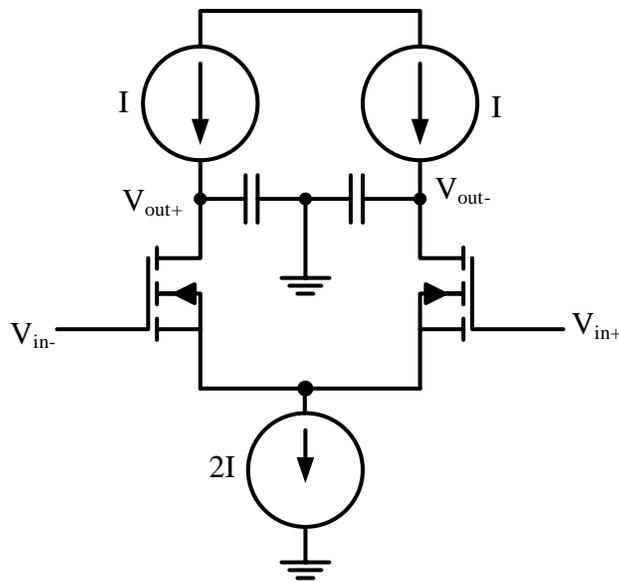
**Fig. 4.10. Differential delay cell with current source loads.**
