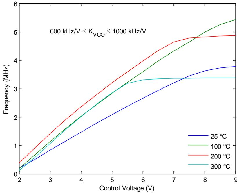
**Fig. 6.9. VCO Transfer Function for tapeout 2.**
