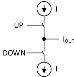
**Fig. 2.10. Functional diagram of the charge pump.**
