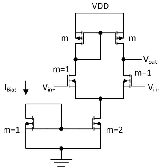
**Fig. 3.21. Difference amplifier schematic used to compare the standard and modified Shichman-Hodges models.  $I_{bias}$  is stated  $I_D$  from the table, and PFET multiplicity,  $m$  is given in the table.**
