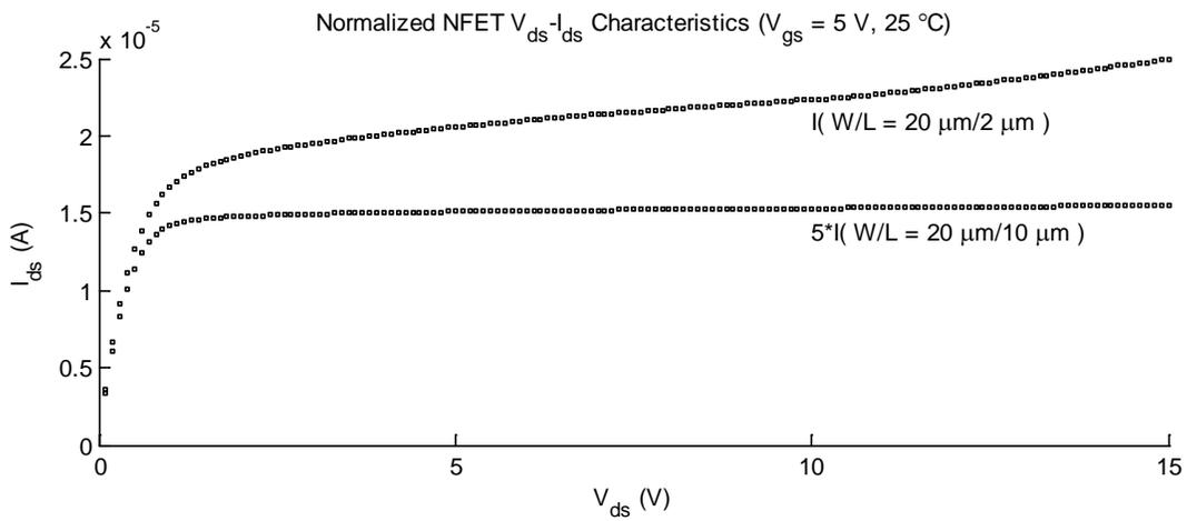
**Fig. 2.4. NFET  $V_{ds}$ - $I_{ds}$  curves normalized for  $W/L$ .**
