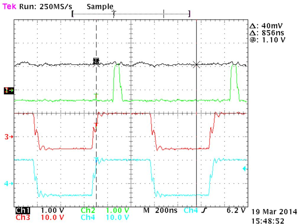
**Fig. 5.4. Transient testing of the PFD at 1 MHz. Ch1 (black) is the DOWN output, Ch2 (green) is the UP output, Ch3 (red) is the DCLK input, and Ch4 (blue) is the CLK input. In this case, the CLK input very slightly leads the DCLK input, and after some delay, the UP output is asserted before resetting. Ch1 and Ch2 are measured by 10x active probes, so the voltage scale is actually 10 V/div, and there is a DC offset (DOWN is always logic 0).**
