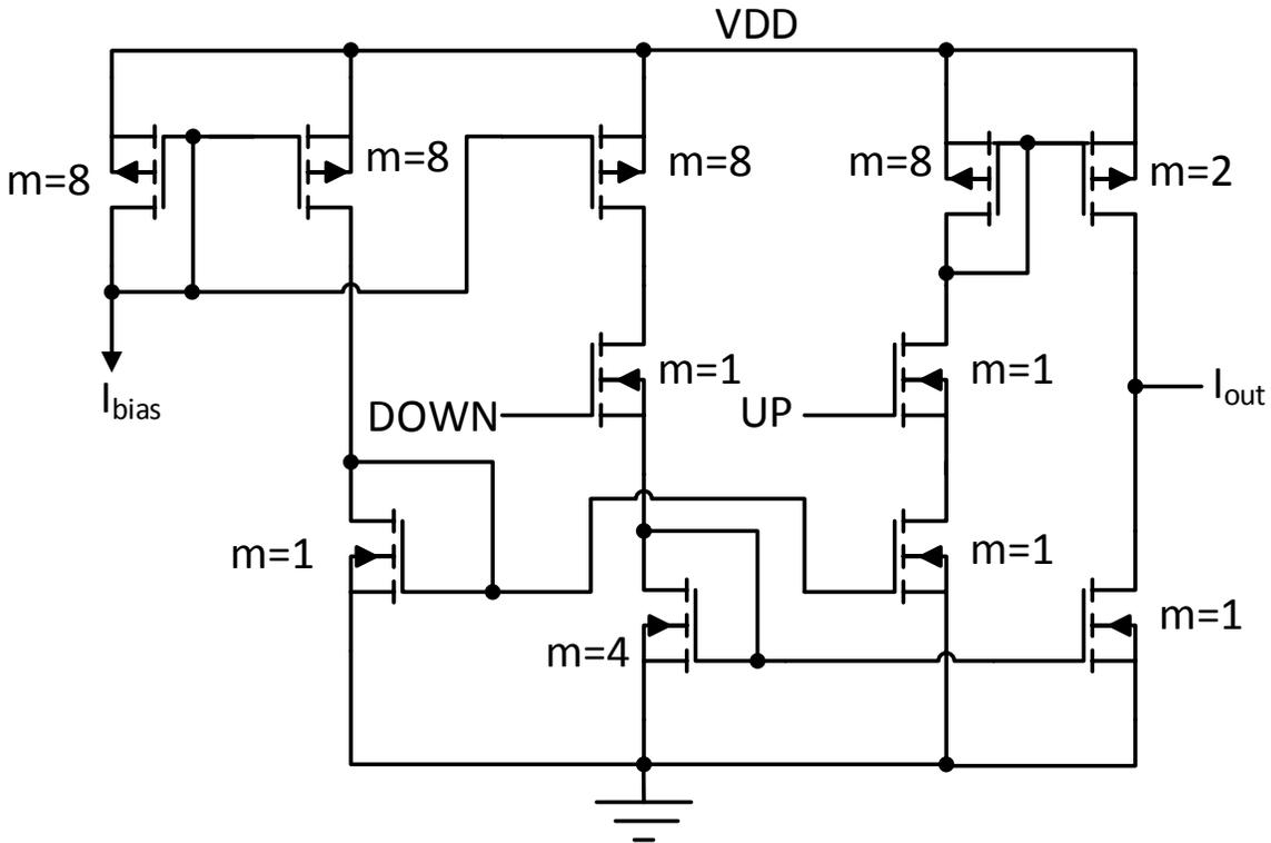
**Fig. 4.7. Charge pump schematic showing device multiplicity.**
