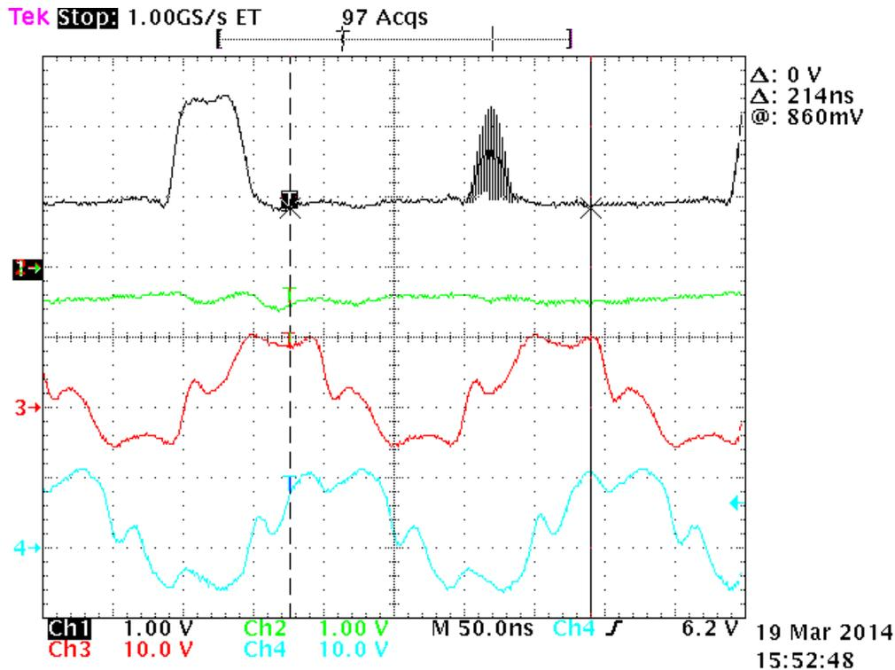
**Fig. 5.6. Transient Testing of the PFD at 5 MHz. Channel assignments are the same as the previous figure. In this case, DCLK input leads the CLK input, and the DOWN output is properly being asserted at one time, but is glitching at another time. The poor quality of the input waveforms is due to reflected waveforms from the PFD input (there is no terminating 50-ohm impedance for matching coaxial inputs).**
