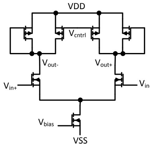
**Fig. 2.15. Maneatis delay cell found in differential VCOs.**
