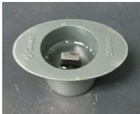
Figure 30 – Epoxy Hardening Container with Sample
