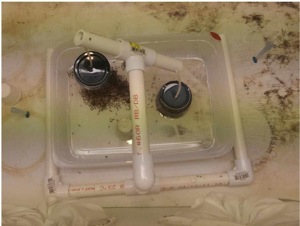
Figure 4.1 Manual cup-lever system used in replications. Cups were alternated by reaching into the quarantine box and rotating the arms of the lever.
