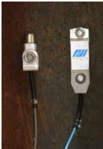
Figure 2.9. Strain gauge and accelerometer attached to a pile for dynamic testing (GRL Engineers, Inc. 2014)
