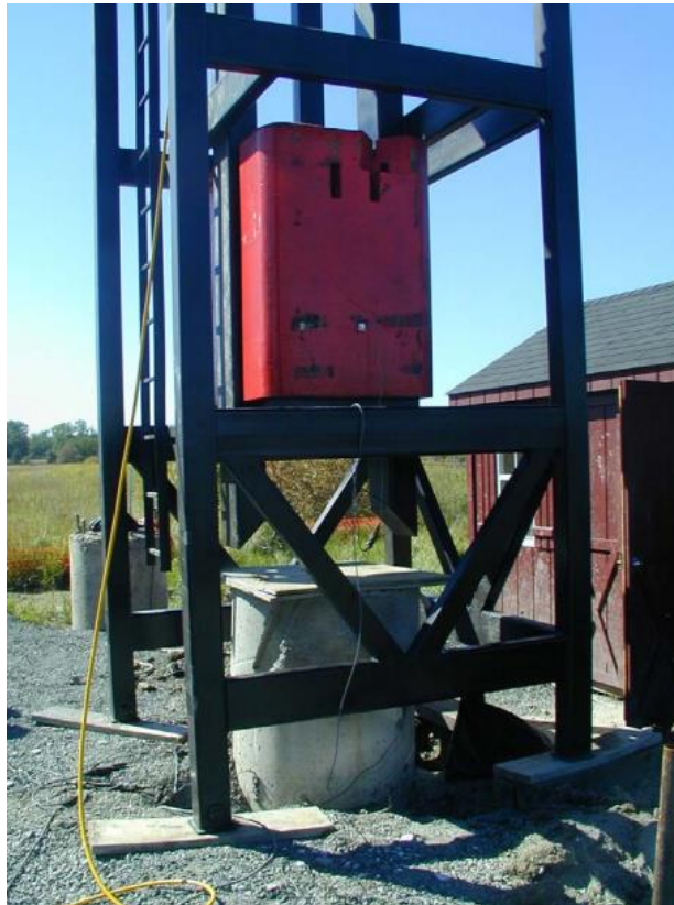
Figure 2.11. Newton's APPLE loading system (PDI 2002)
