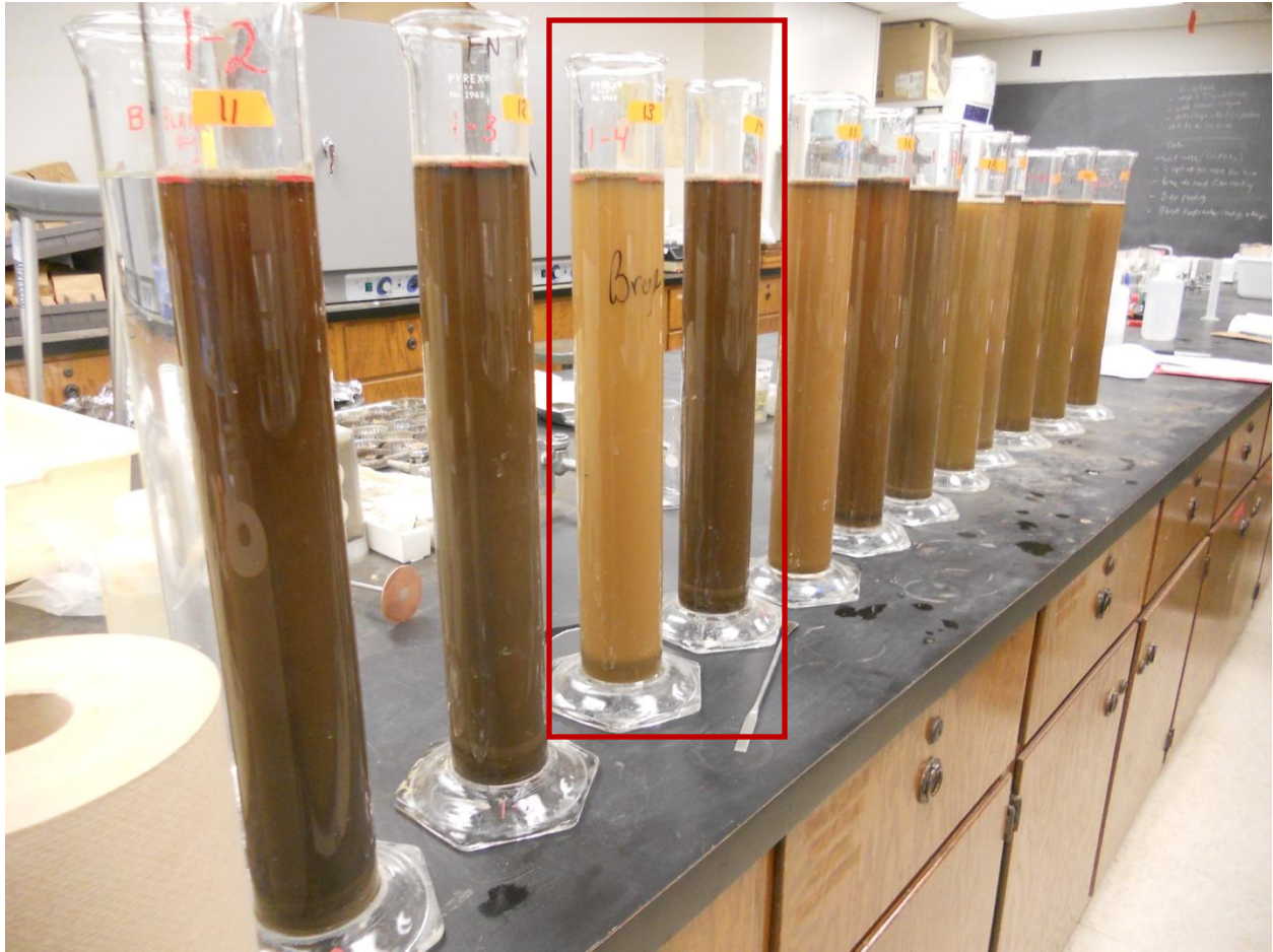
Figure 4.13. Photograph of sedimentation cylinders with incorporated samples. Each pair of cylinders (starting left to right) represents a pair of soils from the same soil type on the soils map, but one is from a highly maintained site, and one is from a minimally maintained site. Pairs 3-4, 5-6, and 7-8 were visibly different in color. The two most different (highlighted by the red rectangle) are sample 3, which is a wheat color, and sample 4 which is much darker.
