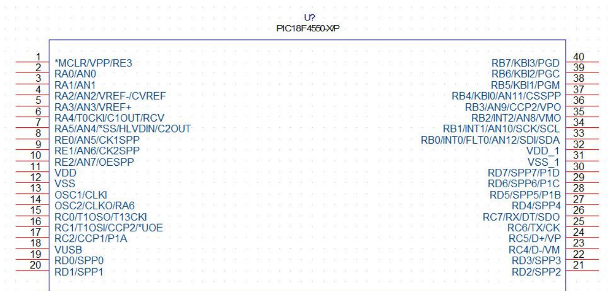
Figure 4.3 – Designed Capture symbol for a 40-pin DIP-type PIC18F4550 micro-controller.
