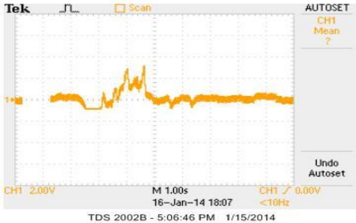
4.5(a): EEG Signal from the gain stage with arm movement.
