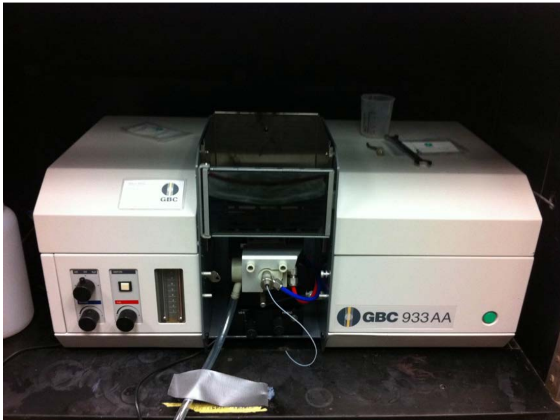
Figure 5: The Atomic Absorption Spectrometers GBC 933 (photo by author)
