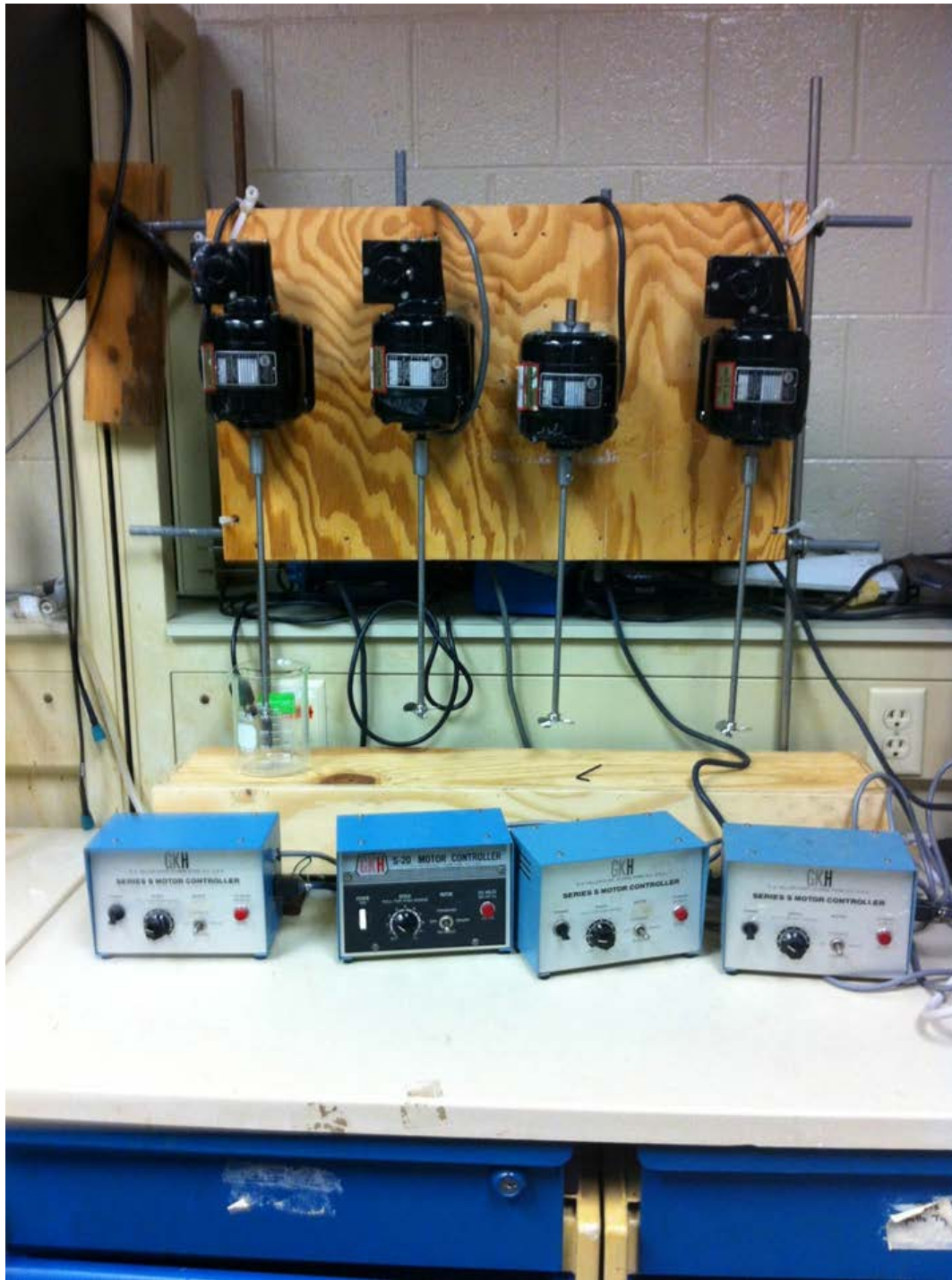
Figure 6: Coagulation Experimental Setup (photo by author)
