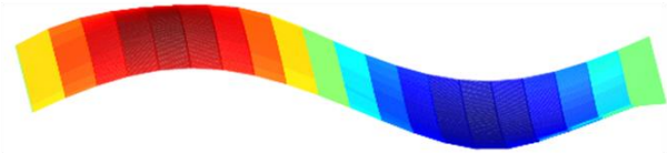
Mode 4: Second Bending Mode (21.7 Hz)
