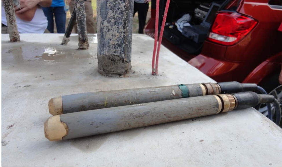
Figure 5.25. Photograph of piezoelectric probes utilized for CSL testing.
