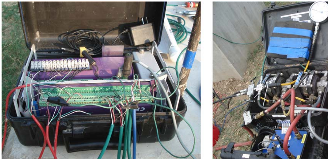
(a) (b) Figure 5.28. Photographs of (a) data acquisition system, and (b) automated pressure regulator and hydraulic pump utilized to perform the O-Cell testing.
