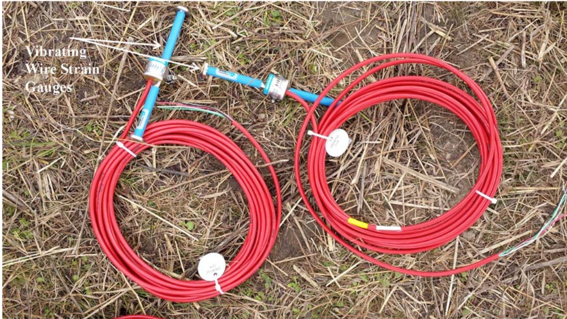
Figure 6.7. Photograph of the linear vibrating wire strain gauges utilized in each shaft.
