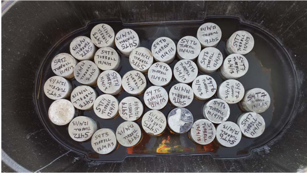
Figure 6.42. Photograph of test shaft T-S4 cylinders prior to transport.
