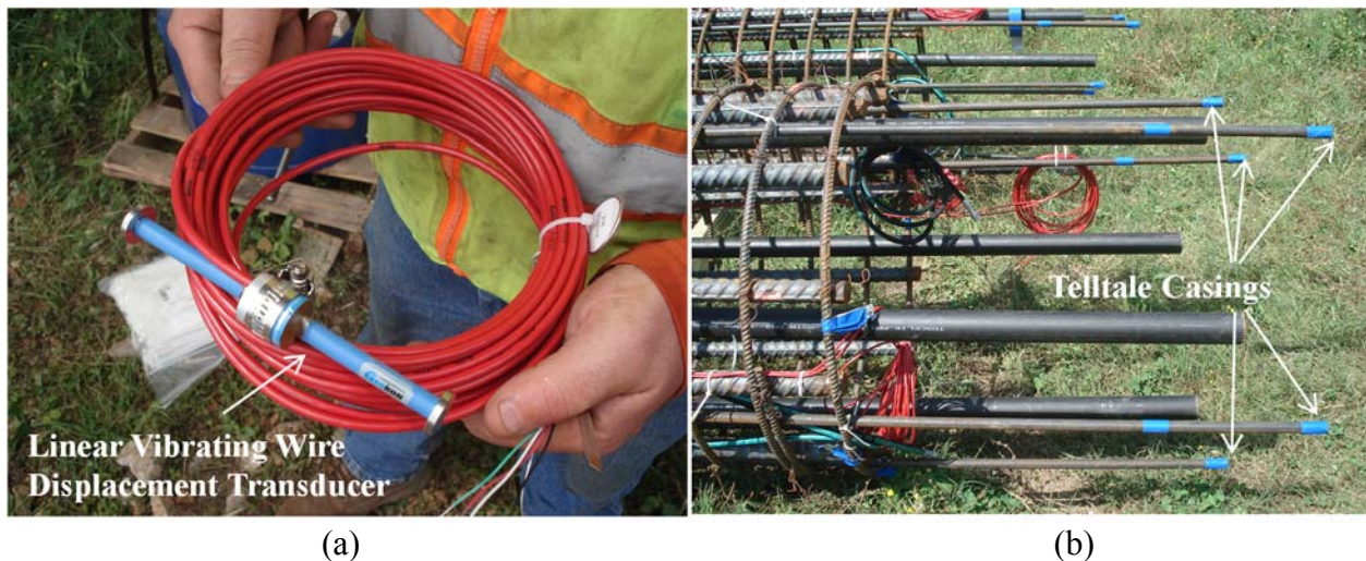
Figure 5.5. Photograph of (a) linear vibrating wire displacement transducers and (b) telltale casings utilized in each shaft.
