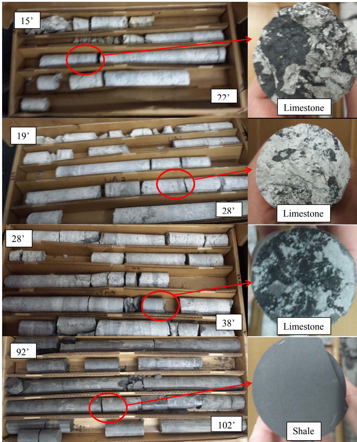
Figure 3.7. Examples of the cores of limestone and shale as collected and stored by researchers at the University of Arkansas.
