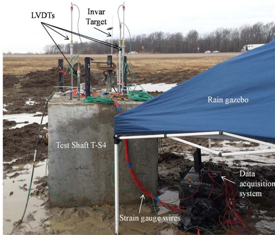
Figure 6.49. Photograph of the test shaft T-S4 O-Cell test in progress.
