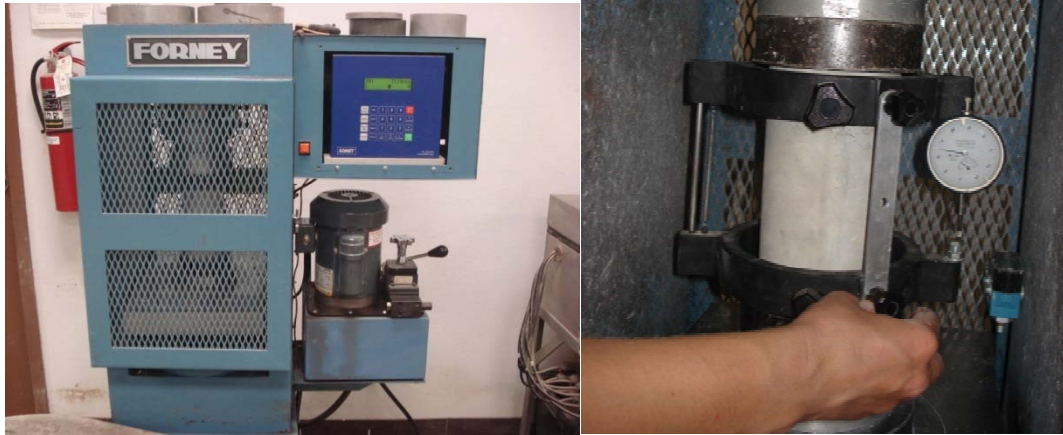
(a) (b) Figure 5.23. Photographs of (a) uniaxial compression testing, and (b) compressometer used for modulus of elasticity testing.
