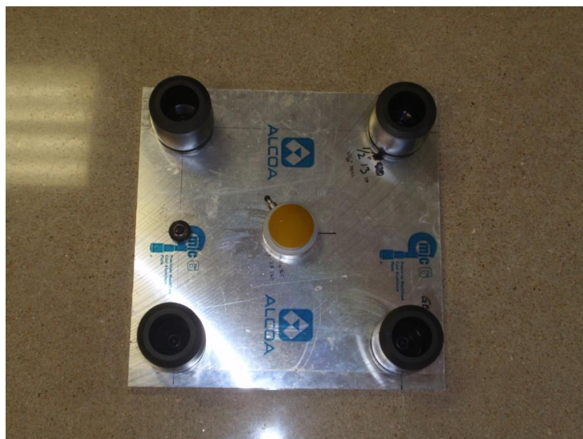
Figure 4.8: Bottom of force plate assembly with TecPak GBA 113S bumpers (corners) and Model 200C50 impact force sensor (center).
