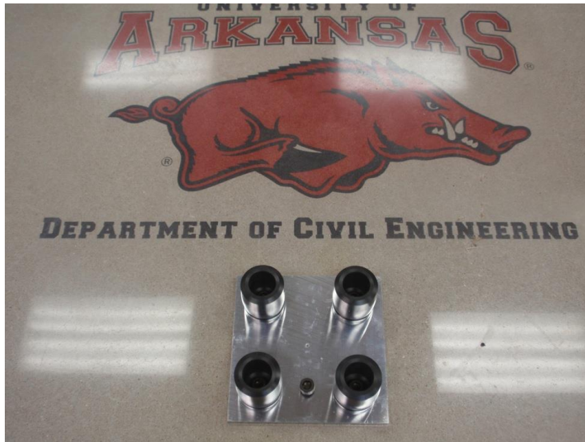
Figure 4.7: Bottom of force plate assembly with TecPak GBA 119S bumpers at corners (impact force sensor not shown)
