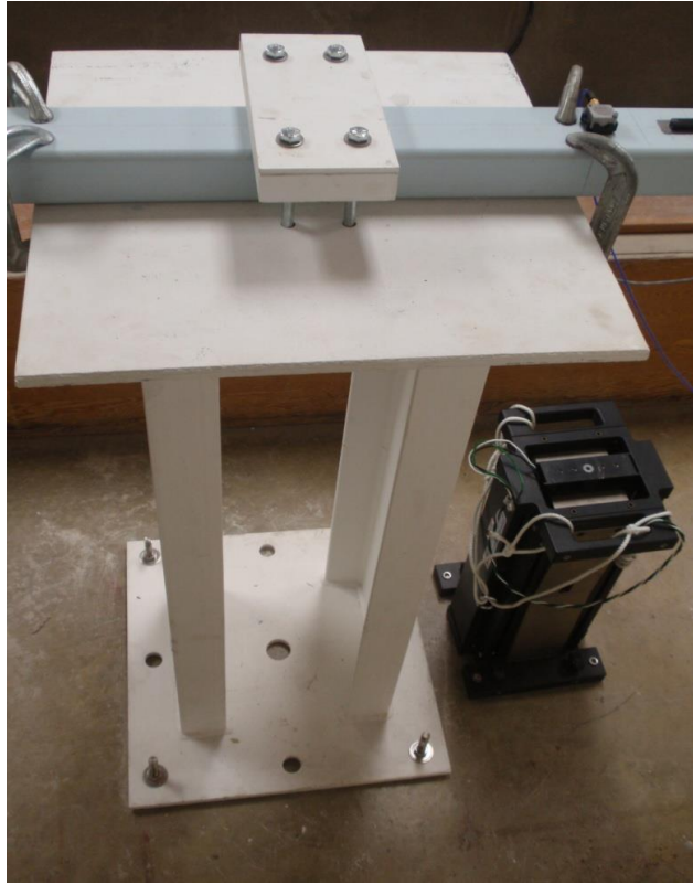
Figure 3.2: Fixed end of HSS cantilever
