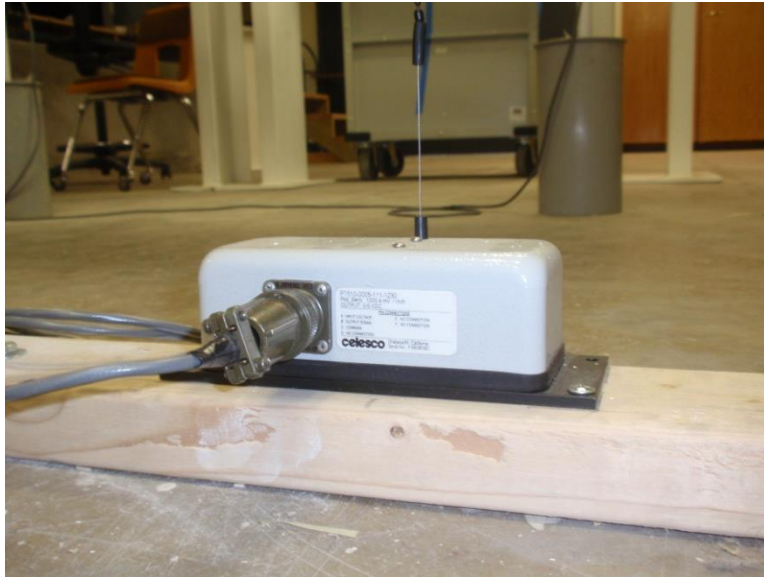
Figure 3.13: Photograph of PT-510 string pot installed under the grid model structure. Photo Taken by Jason Herrman, Fall 2010 Engineering Research Center
