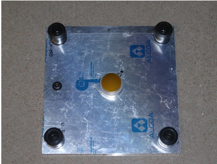
Figure 4.9: Bottom of force plate assembly with TecPak GBA 107S bumpers (corners) and Model 200C50 impact force sensor (center). Photo taken by Jeremy Rawn, Fall 2010 Engineering Research Center
