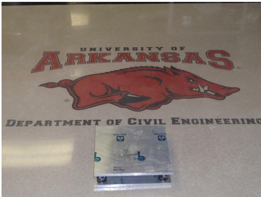
Figure 4.10: Force plate assembly (TecPak GBA 107s bumpers) with top aluminum plate installed. Photo taken by Jeremy Rawn, Fall 2010 Engineering Research Center
