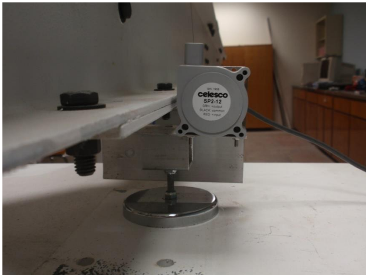
Figure 3.11: TML CDP-25 displacement transducer installed under the grid model structure. Photo Taken by Jason Herrman, Fall 2010 Engineering Research Center
