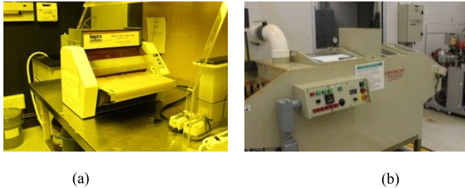
Fig. 6.1 Kepro bench-top laminator (a) and chemicut machine for etching (b) (photo by author)
