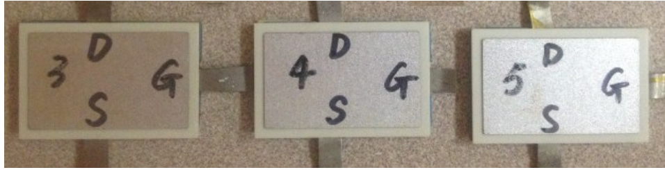
Fig. 8.21 Power modules for thermal cycling experiment (photo by author)
