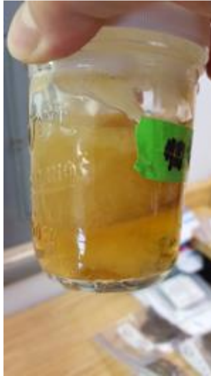
Figure 2 Image of a finished mycelium culture grown in a solution 4% light malt extract at a temperature of 27°C to be used as inoculum for the fungal growth experiments. The liquid in the jar is the growth medium and the fibrous cotton-like substance in the jar is the mycelium.
