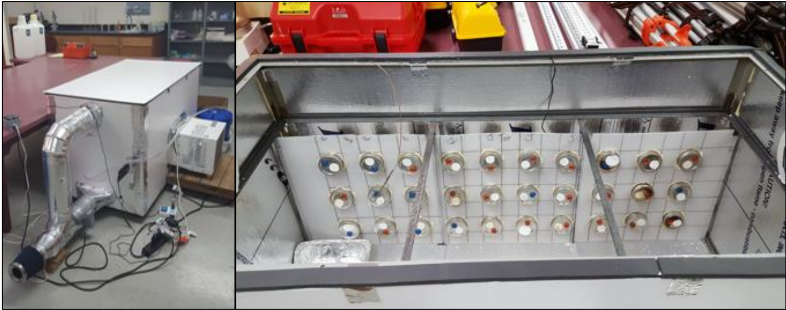
Figure 4 Images of the external (left) and internal (right) of the mushroom growth chamber. The image of the internal of the chamber also shows jars in the mushroom rack, which would contain the substrate and the mushroom would grow out of.
