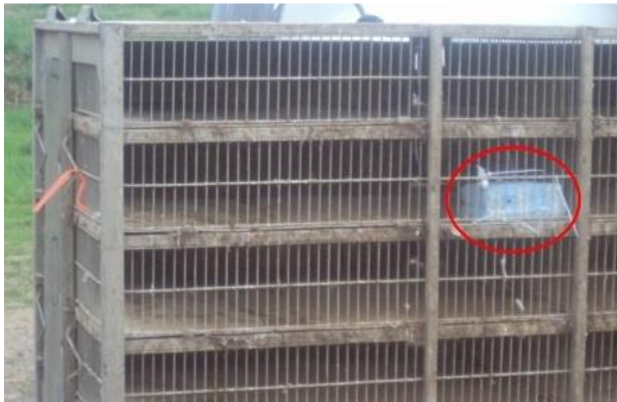
Figure 3.8: Electronic chicken installed on the middle back of a module during commercial live-haul transportation.
