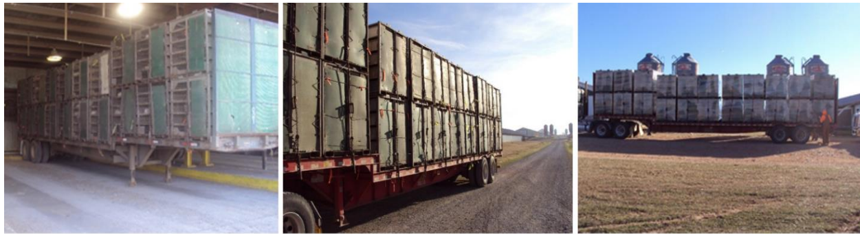
Figure 3.3: (A) Trailer with Boarded-Single configuration kept in the holding shed (B) Trailer with Boarded-Double configuration during winters (C) Trailer with Boarded-Wrapped configuration during extreme winters.
