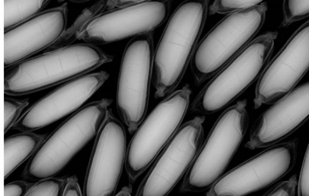
Figure 4. X-ray images of rough rice kernels at 1X, 2X, 3X, 4X, 5X, and 6X magnifications. Each image contains the same set of rice kernels.
