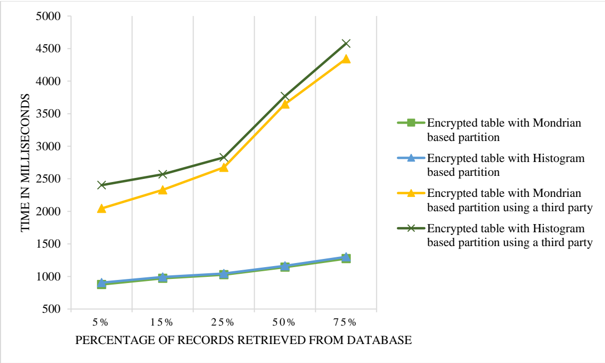
Figure 4.3. Response times for data retrieved from a table having 100,000 records with record size 78 bytes using Mondrian and Histogram based partition
