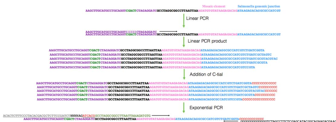
Figure S2.2. Tn-seq library preparation diagram for Illumina sequencing. The genomic DNA extracted from the selected library and subjected to two PCR amplifications. First PCR was linear and specific forward primer used to capture and amplify Tn5 junctions. Second PCR was exponential and Illumina adaptors with a barcode added. The PCR product gel purified and sequenced on an Illumina platform.
