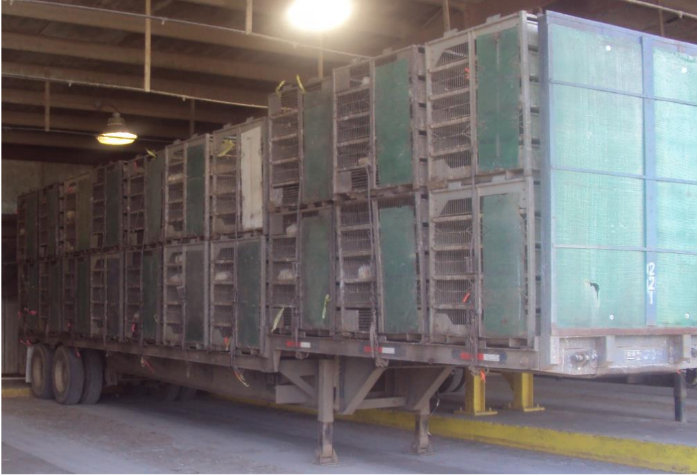
Figure 4. Industry standard drop deck poultry transport. Modules have single side boards for reduced air flow in cool weather conditions (2.4 to 21.0 °C).
