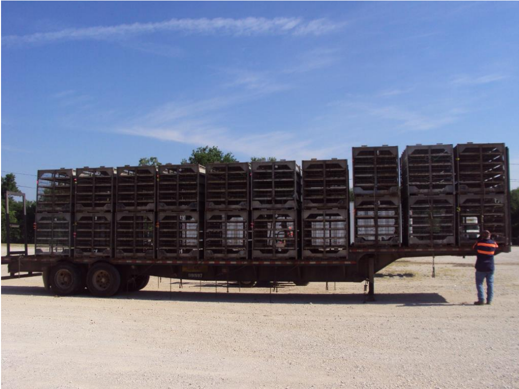
Figure 5. Open sided modules for use in moderate temperatures and high temperatures (19.3 to 29.1 °C)
