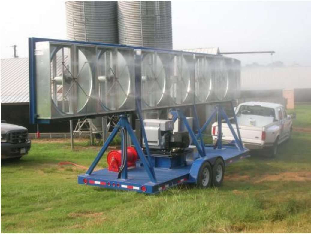
Figure 6. A fan trailer equipped with spray nozzles used for heat mitigation while the trailer is being loaded on the farm.
