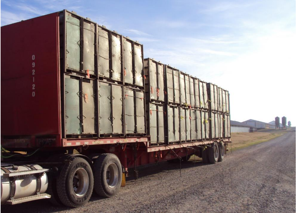
Figure 3. Double side boarded modules for reduced air flow in cold weather (-16.4 to 10.4 °C)
