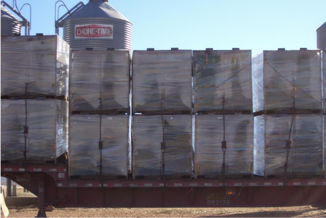
Figure 2. Modules after being loaded with broilers, wrapped with plastic and loaded on to the transporter. Plastic wrap is used only in extremely cold conditions (-15.8 to 2.8°C)
