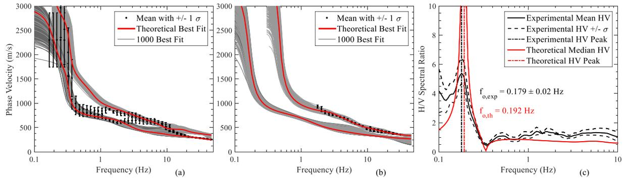
Figure 5. Experimental dispersion data and theoretical fits for the 1000 lowest misfit  $V_s$  profiles at the TPLC site, (a) Rayleigh wave and (b) Love wave. (c) Experimental HVSR curve and theoretical HVSR curve for the median of the 1000 lowest misfit  $V_s$  profiles at the TPLC site.
