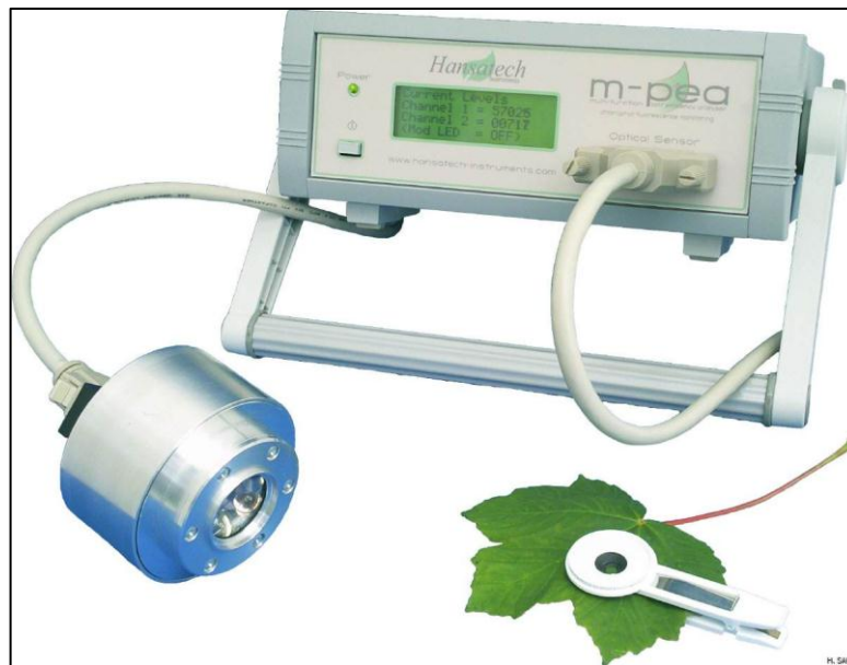
Plate 1. Instrument used to measure fluorescence showing the chlorophyll fluorescence data logger, the sensor, and the leaf clip for dark adaption.
