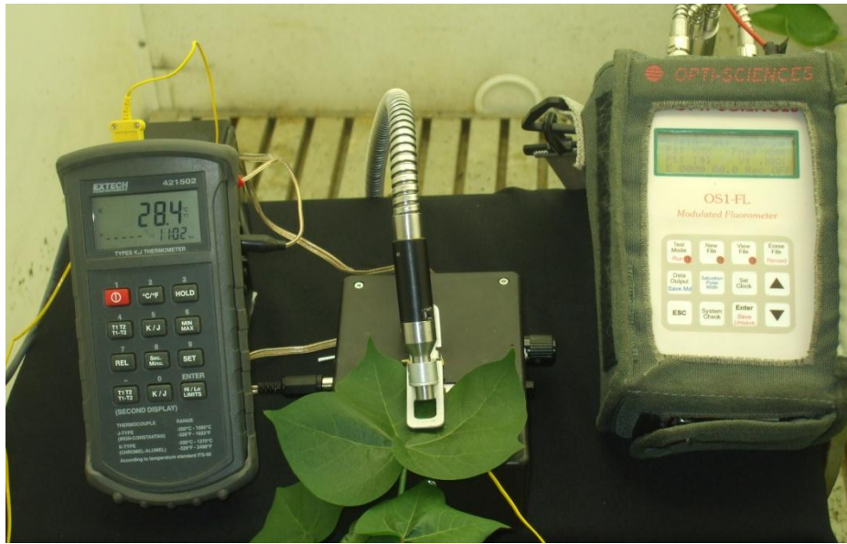
Plate 1. Leaftech instrument with digital thermometer, leaf clip holder and cotton plants and fluorometer.
