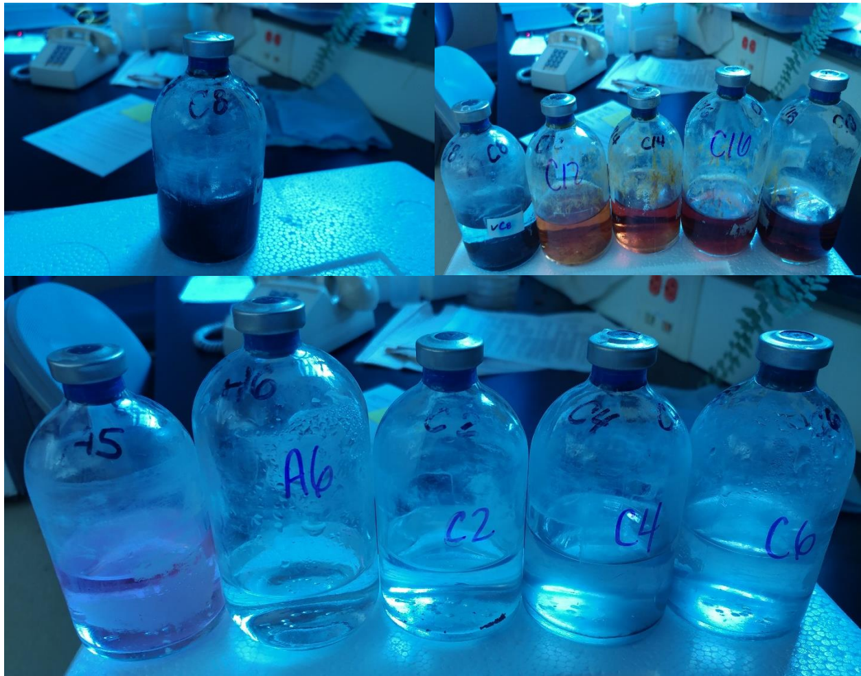
Figure 10. Samples of sulfate reducers producing sulfide (black precipitate) as part of their metabolic activity (sulfate anaerobic respiration).
