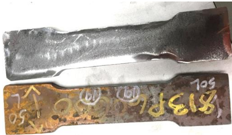
Figure 31. Corroded (bottom) and uncorroded (top) steel surfaces
