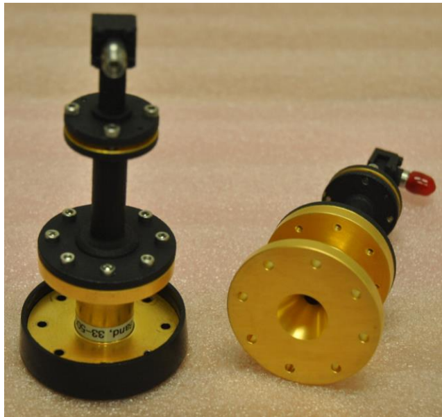
Figure II.11. B-band transitions with 1.85 mm coaxial connectors.
