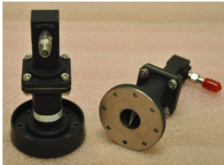
Figure II.8. Ku-band transitions with 3.5 mm to 1.85 mm coaxial adapters.
