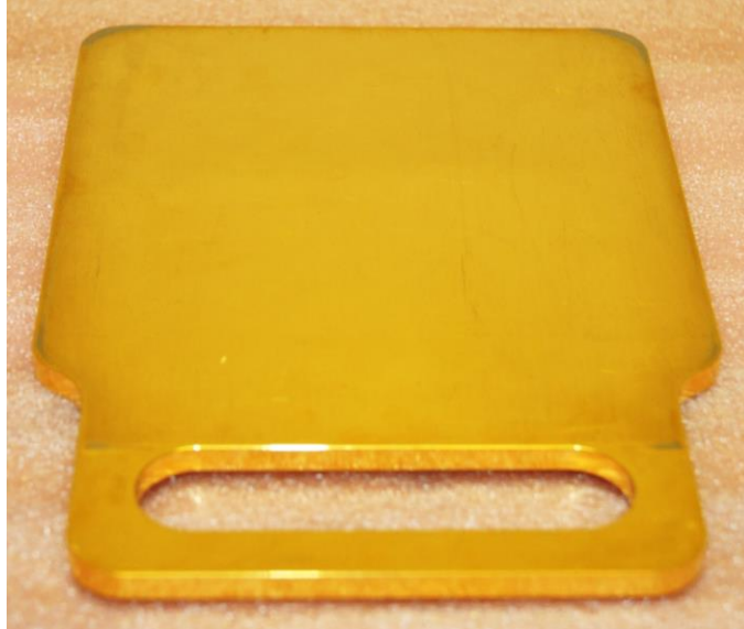
Figure II.21. Gold-plated reflective plate used for TRL calibration.
