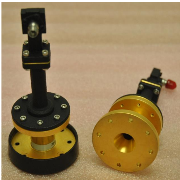
Figure II.10. Ka-band transitions with 1.85 mm coaxial connectors.
