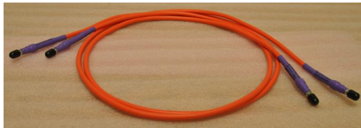
Figure II.3. MegaPhase RF Orange Bench Test cables.
