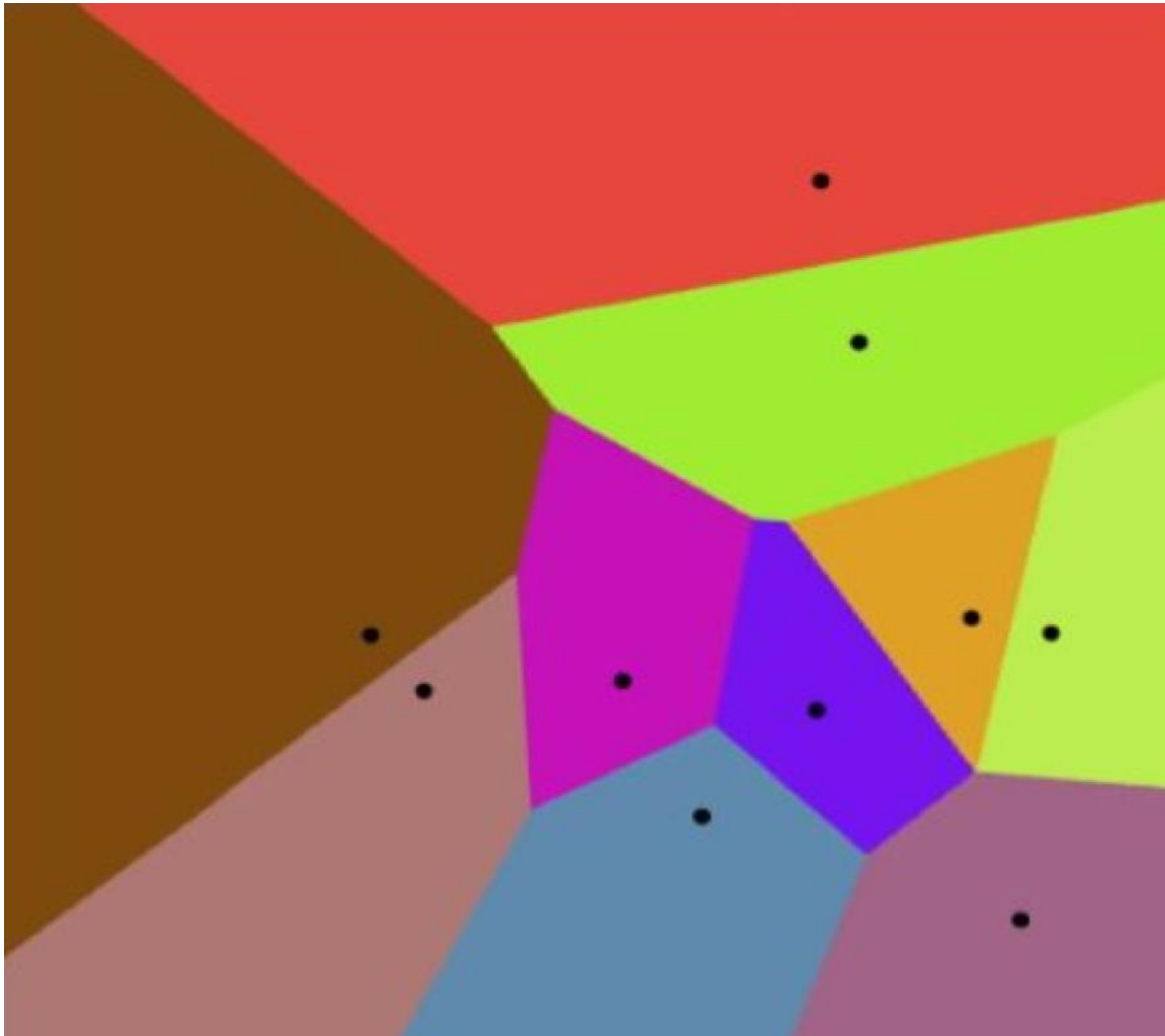
Figure 6. Illustration of Voronoi diagram. Black dots are called localizations or seeds. Colored regions are called Voronoi cells.
