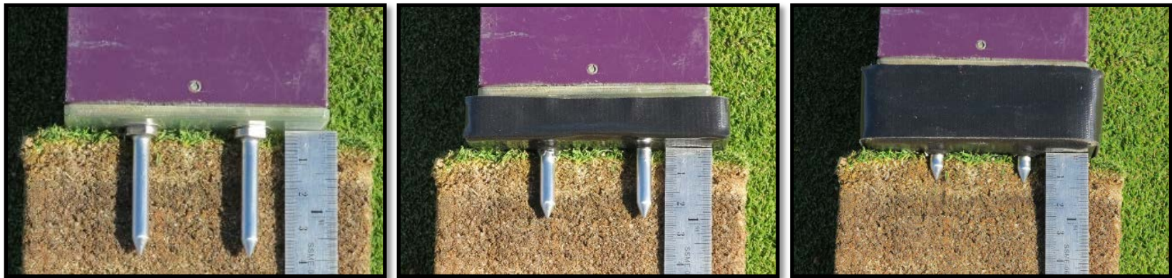
Fig. 1. a: FieldScout TDR300 using Turf rods for standard 3.8 cm measurement depth. b: FieldScout TDR300 using Turf rods fit with spacer-block to achieve 2.5 cm measurement depth. c: FieldScout TDR300 using Turf rods fit with spacer-block to achieve 1.2 cm measurement depth.
