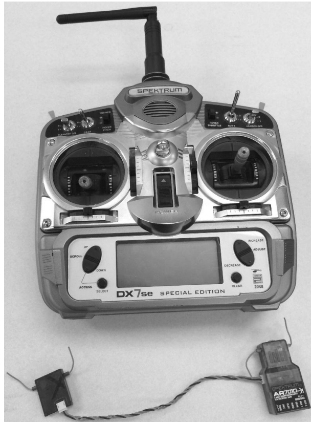
Figure 7. Spektrum DX7SE Transmitter and AR7010 Receiver
