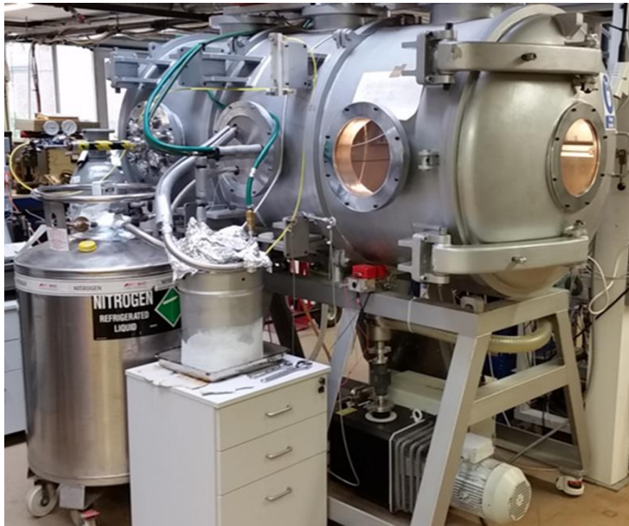
Figure 3.2. The Large Mars Planetary Environmental Simulations Chamber (centre), vacuum pump (bottom), liquid nitrogen supply (left) and CO 2 gas cooler (front left of centre).
