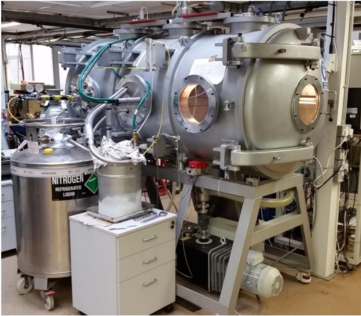
Figure 2.4. Mars Chamber (center), vacuum pump (bottom), liquid nitrogen supply (left), CO 2 gas cooler (front left of center).
