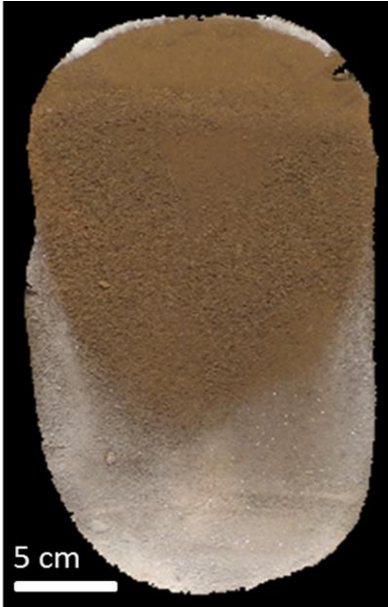
Figure 2.7. Orthophoto of the regolith surface at start of sublimation for Run 1. Slope crest is at the top of the image. The width of the test section is 30 cm.
