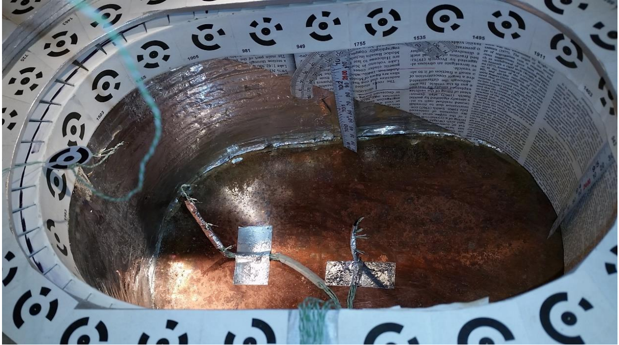
Figure 4.12. Thermocouple placement inside the copper coiled box for Sets IV-VI. The mid-slope thermocouple tree, with three bundled type K thermocouples, is taped to the middle of the box bottom. The larger, rear thermocouple tree has five bundled type K thermocouples. At the far left of image, a single type K thermocouple is affixed to a coded photogrammetric target. This was placed on the surface of the slope. This is a typical arrangement, although for some runs a thermocouple was affixed ~1 cm above the box bottom near the toe of slope (far right in the image).
