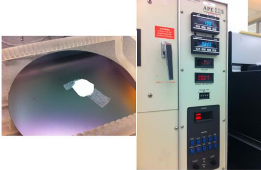
Figure 5.11. Oxygen plasma instrument used to chemically modify the surface of PDMS replicas and PES filters (left side). APE-110 - Automated Plasma Cleaning System (600 mTorr, 100 W).
