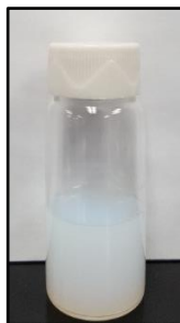
Figure 2.4. Zinc oxide nanoparticles are dispersed in 1-butanol for spin coating application. “Photo by Ramesh Vasan”
