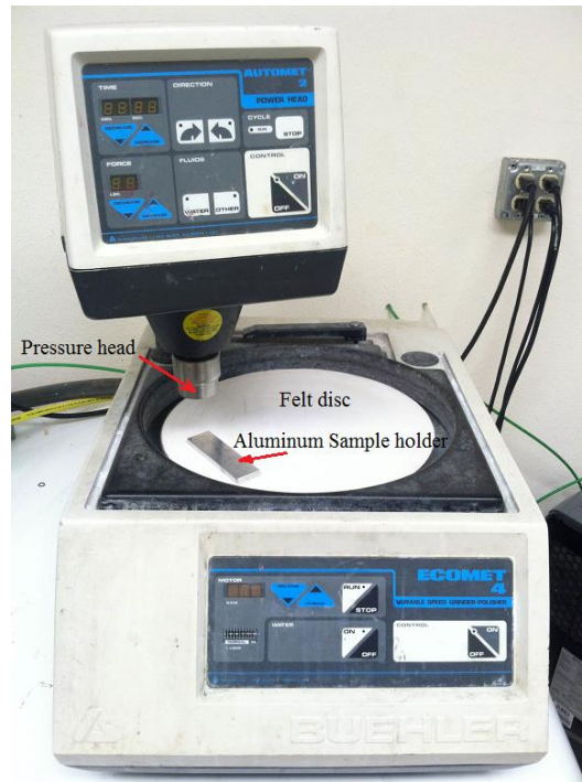
Figure 3.17 Abrasion test setup
