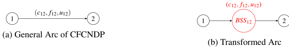
Figure 3: Transformation of each arc of fixed charge network design problem to our research problem.
