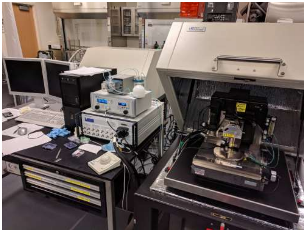
Figure B.2. Photo of Veeco Dimension V AFM (taken by author).
