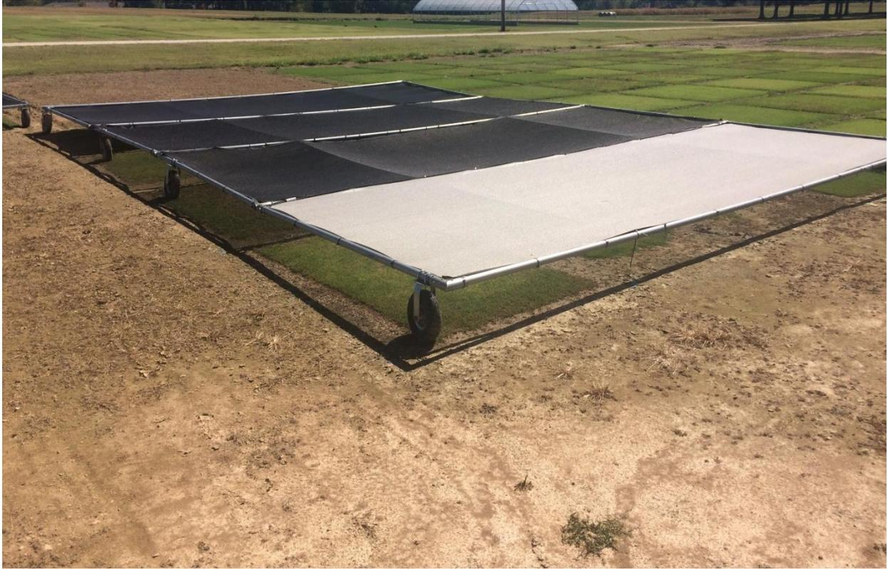
Figure 3.1. Shade structure system utilized to apply various shade intensities to four turfgrass types.
