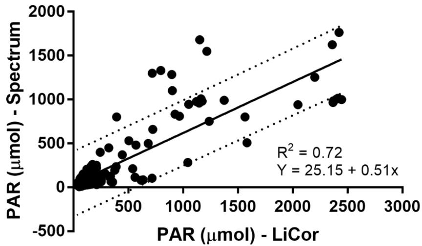
Figure 4.2. Linear regression model to evaluate accuracy of a Spectrum LightScout quantum light meter to measure PAR light compared to measurements obtained from LI-COR 1-m line quantum light meter under shade canopies of six tree species. Dashed lines represent 95% prediction intervals.
