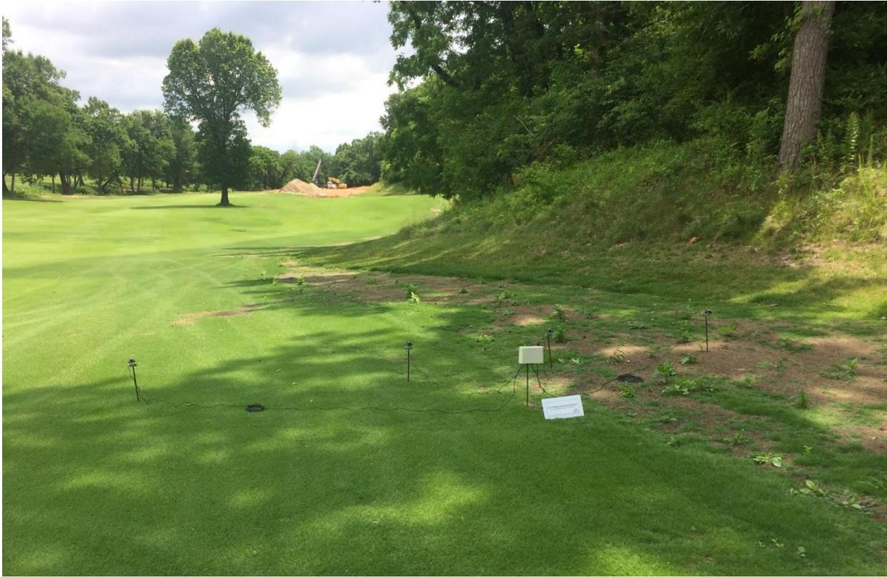
Figure 3.2. Quantum light sensors placed along a line transect perpendicular to shade damage in the following positions: 1) area of full turfgrass coverage, 2) slight turfgrass decline, 3), extensive turfgrass decline, and 4) complete turfgrass failure.
