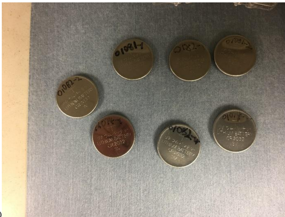
Fig. 4.7. CR2032 button cells: a) negative electrode side, and b) positive electrode side.
