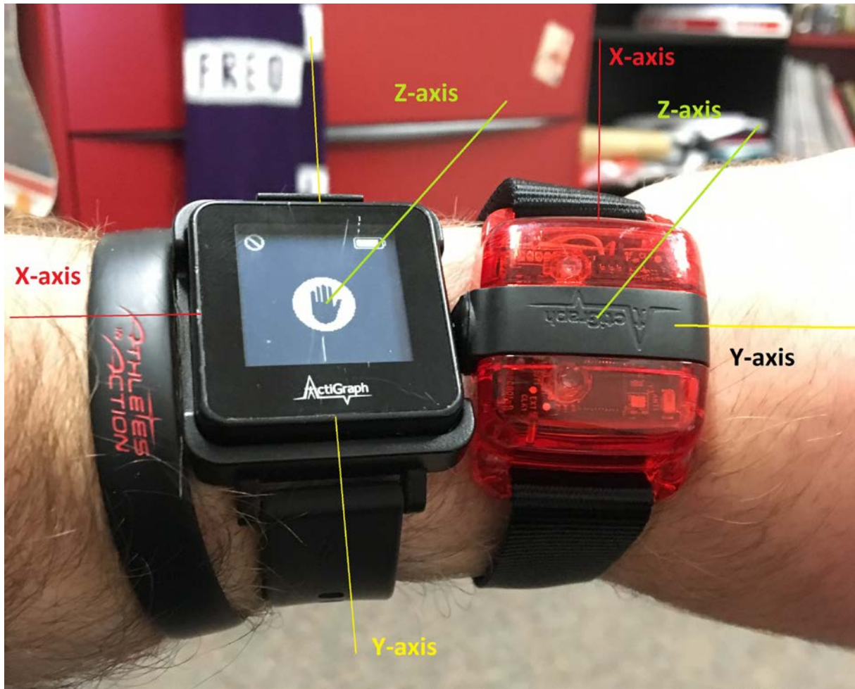
Figure 1. A picture of the Link (left) and GT3x-bt (right) and their axes on the wrist.
