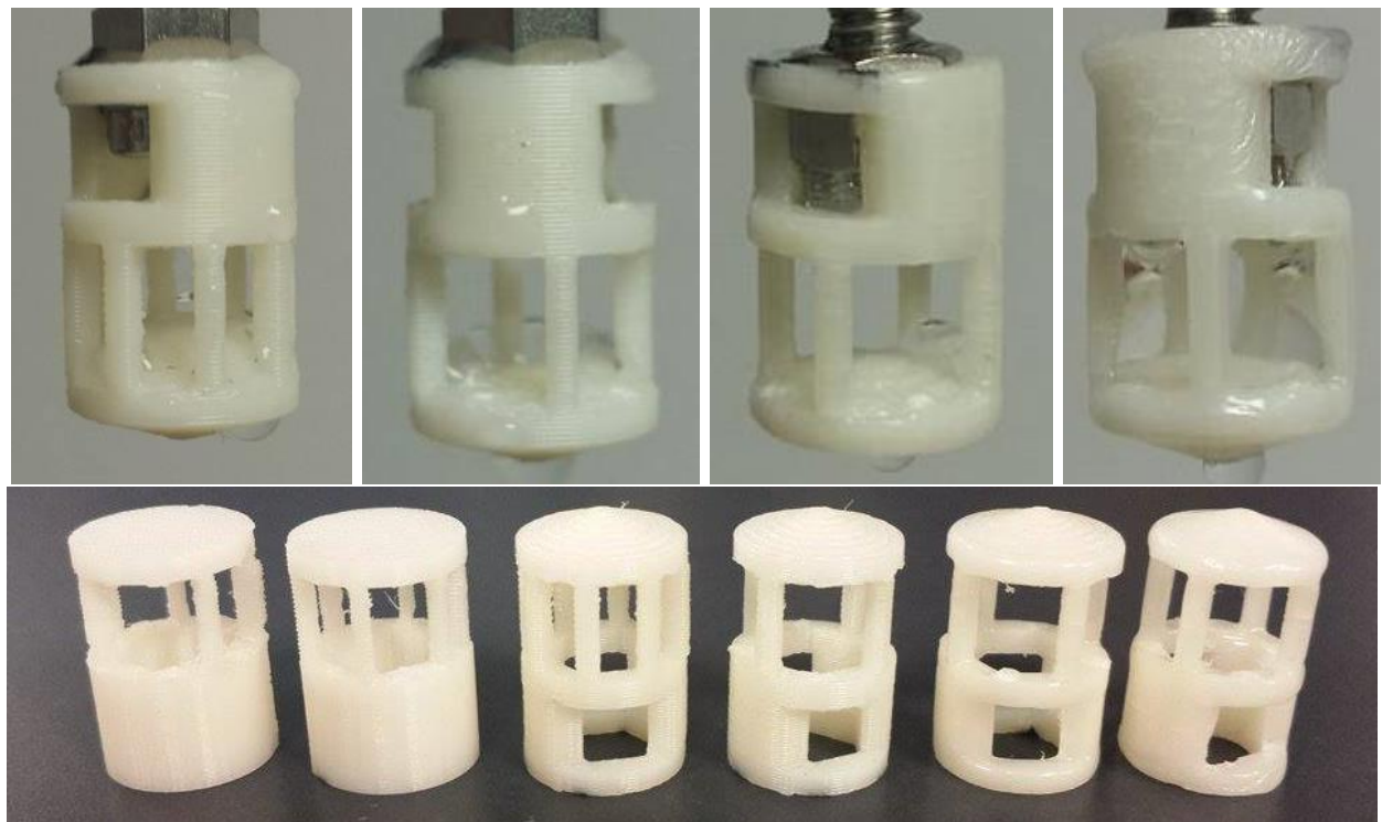
Figure 101: Filters designed to prevent fluid collection aimed to prevent water blockage
