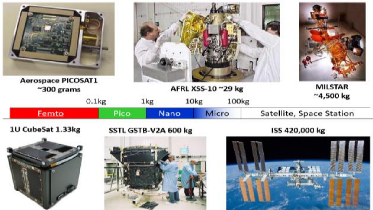
Figure 1: Well-known satellites are typically on the micro/macroscale, but advances in technology have decreased the form factor necessary to conduct high impact space research. Advances in technology, particularly micro/nanotechnology, have further decreased the size of satellites to a handheld size. (Huang, Wilson, & Chan, 2014)
