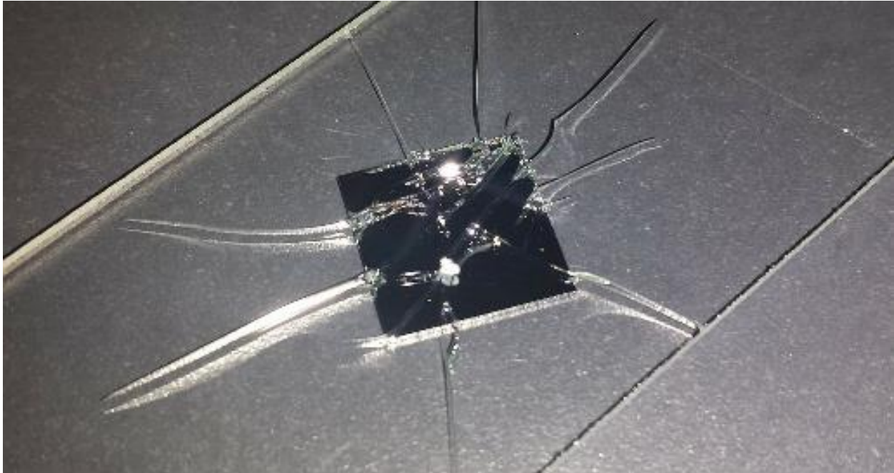
Figure 135: Mismatched coefficients of thermal expansion result in fracture of bonded glass.
