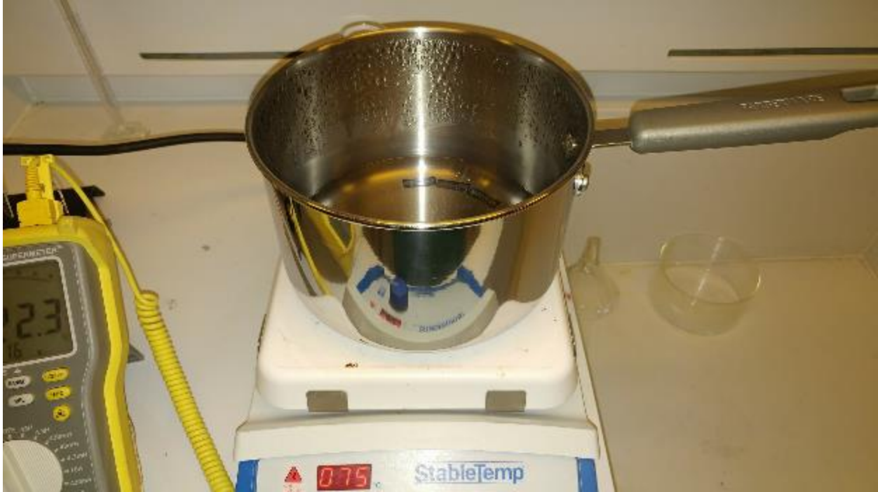
Figure 24: Potassium hydroxide (KOH) etches silicon on the {111} atomic plane. Silicon oxide formed the mask, leaving exposed silicon susceptible to KOH etching, which formed the micro/nanochannels.
