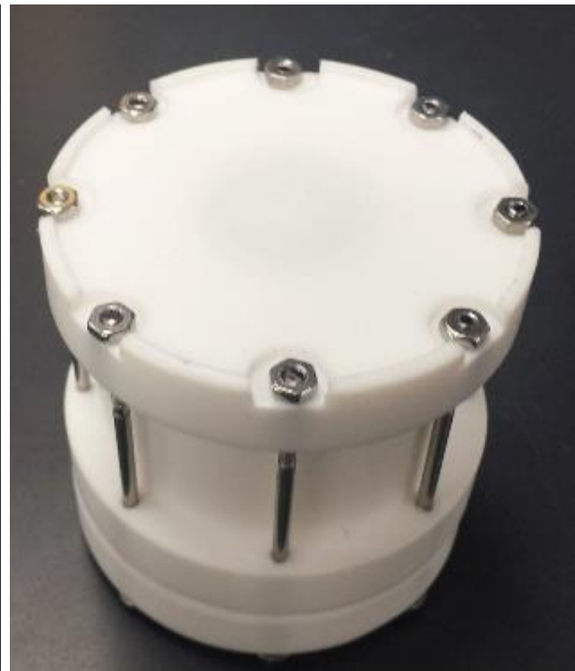
Figure 35: A Teflon propellant test chamber minimized error by limiting leaks and heat loss. Convection is minimal in a vacuum environment and conduction was limited by machining the bottom of the tank, leaving minimal stand-offs to conduct heat.
