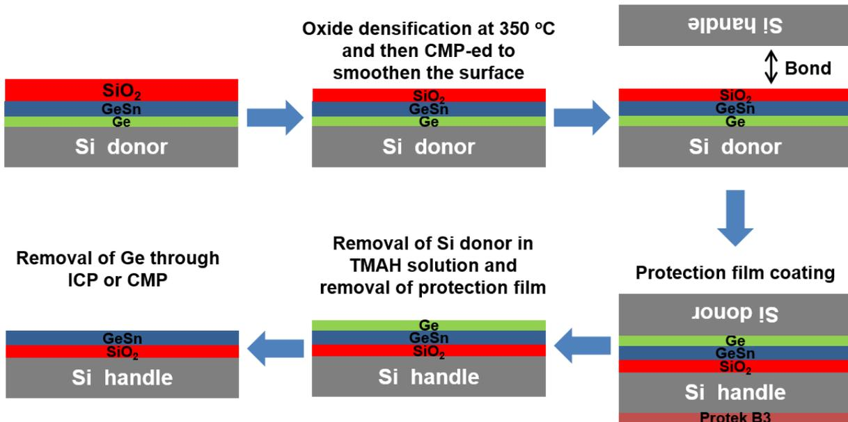
Figure 58: Processing flow of substrate removal process
