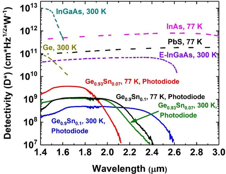
Figure 32: Spectral  $D^*$  of 7 and 10 % Sn photodiodes measured at 0.1 V reverse bias voltage across a 250  $\mu\text{m}$ -diameter device. Other market dominating detectors in same spectral range are plotted for comparison.
