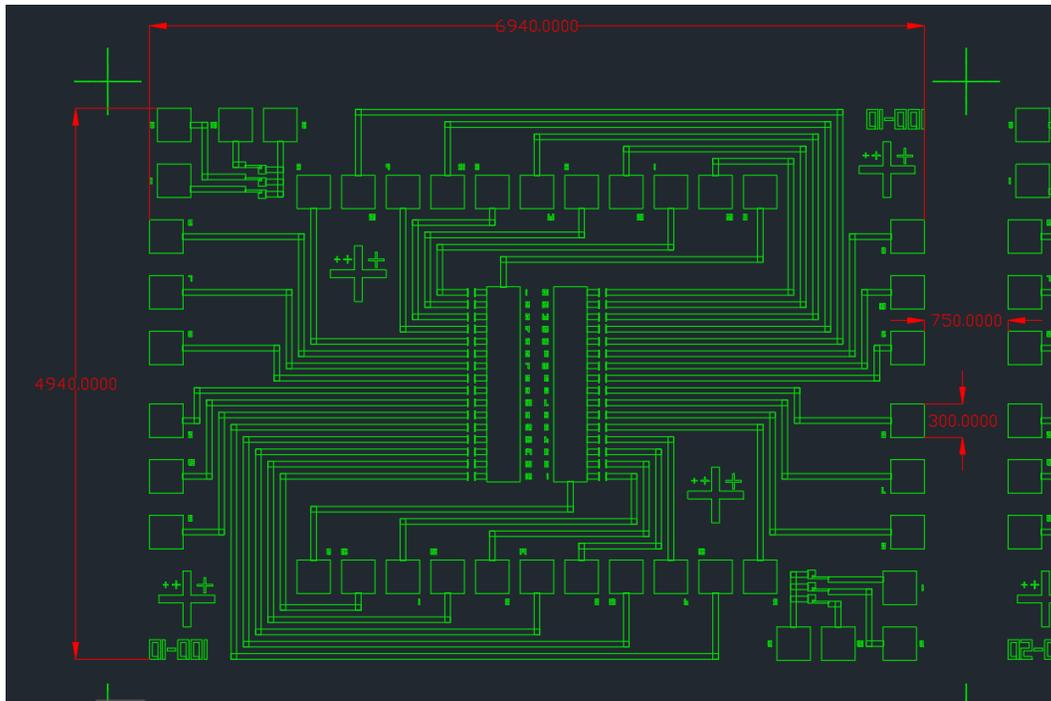
Figure 59: Mask layout (3<sup>rd</sup> mask) of linear array detector.
