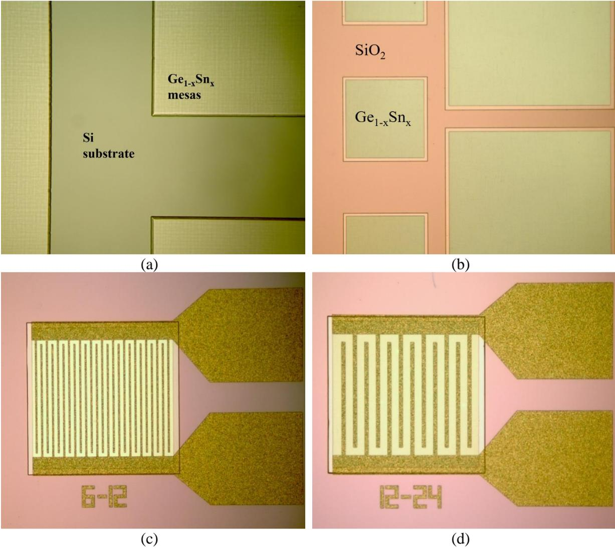
Figure 16: Top view microscope image of (a) ASM 108 after wet etching at low temperature, (b) ASM 108 after defining the active windows, (c)  $500 \times 500 \mu\text{m}^2$  ASM 108 with 6-12 interdigitated electrodes structure after lift-off, and (d)  $500 \times 500 \mu\text{m}^2$  ASM 108 with 12-24 interdigitated electrodes structure after lift-off
