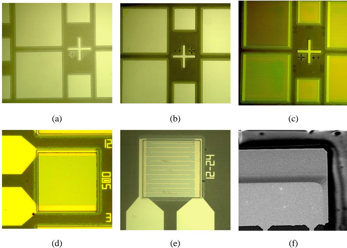
Figure 6: Top view microscope images of (a) mesas etching using RIE (1<sup>st</sup> mask), (b) defined active area with BCB (2<sup>nd</sup> mask), (c) defined metal contacts (3<sup>rd</sup> mask), (d) standard photoconductor after lift-off, (e) 12-24 interdigitated photoconductor after lift-off, and (f) top view SEM image of a metal covered slope created by BCB.
