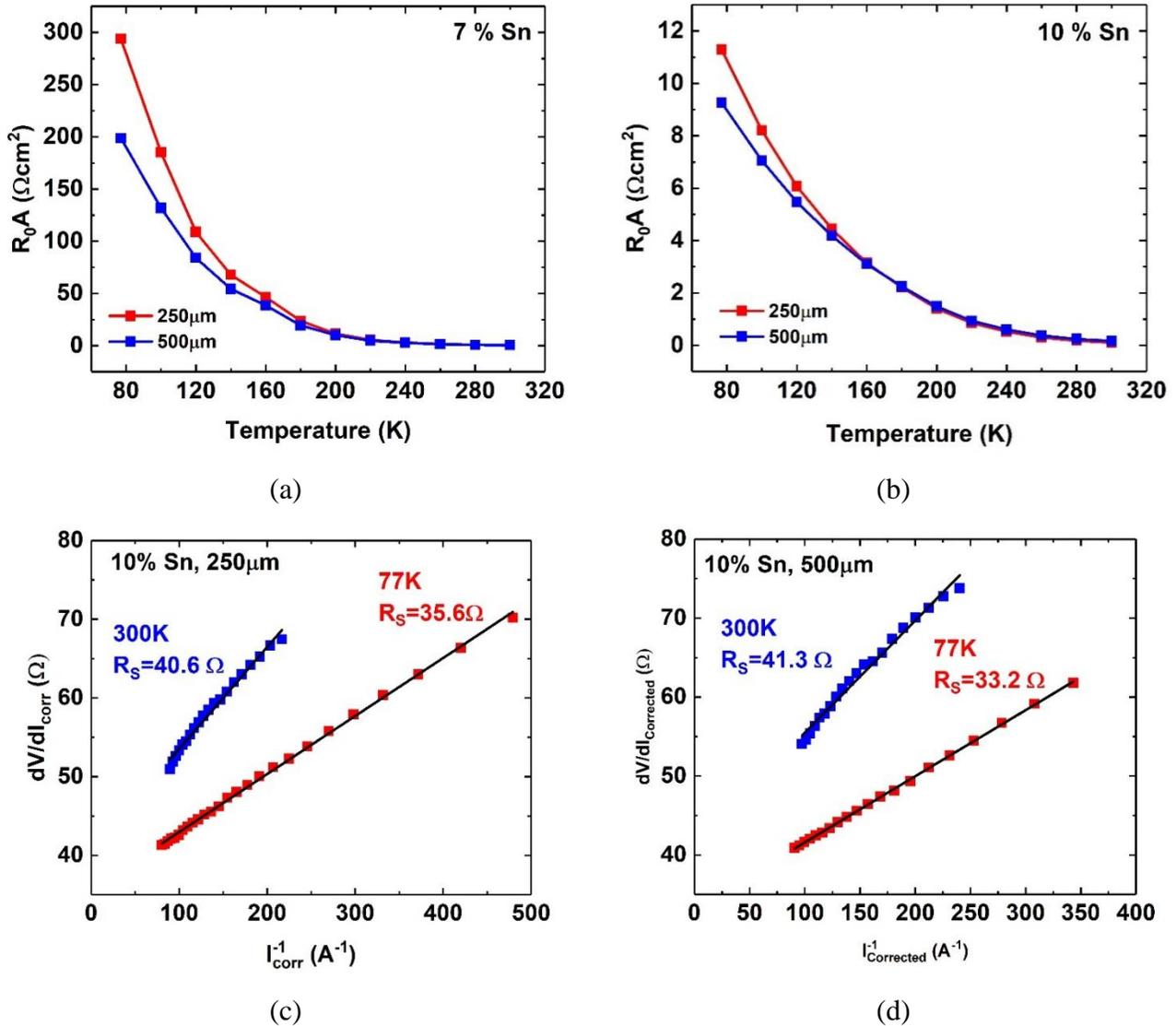
Figure 28: Zero-bias resistance-area product ( $R_0A$ ) at different temperatures of (a) 7 % Sn and (b) 10 % Sn devices. Linear fit of  $(I_{corr})^{-1}$  as a function of  $dV/dI_{corr}$  at 77 and 300 K of the (c) 10 % Sn sample of 250  $\mu\text{m}$ , (d) 500  $\mu\text{m}$  in diameter, and (e) 7 % Sn sample of 250  $\mu\text{m}$  and 500  $\mu\text{m}$  in diameter. Activation energy of 7 and 10 % Sn with different mesa sizes was shown in Figure 28 (f).
