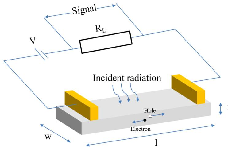
Figure 3: Geometry and bias of a photoconductor
