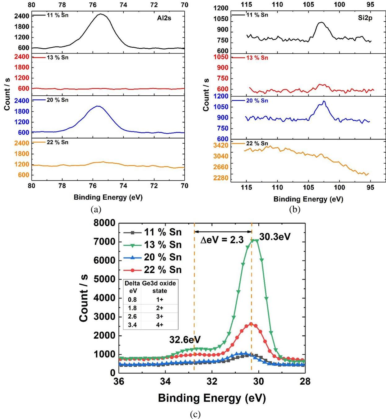
Figure 49: (a) Al<sub>2s</sub> spectra, (b) Si<sub>2p</sub> spectra, and (c) Ge<sub>3d</sub> spectra of 11 %, 13 %, 20 %, and 22 % Sn samples after wet etching in BOE solution for 15-17 s. The small shift towards longer binding energy level in (c) signals the existence of germanium oxide.
