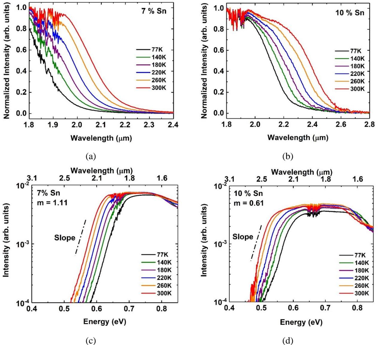
Figure 29: Normalized temperature dependent spectral response of (a) 7 % Sn photodiode and (b) 10 % Sn photodiode. Temperature dependent absorption edge of (c) 7 % Sn photodiode with  $m = 1.11$  and (d) 10 % Sn photodiode with  $m = 0.61$ .
