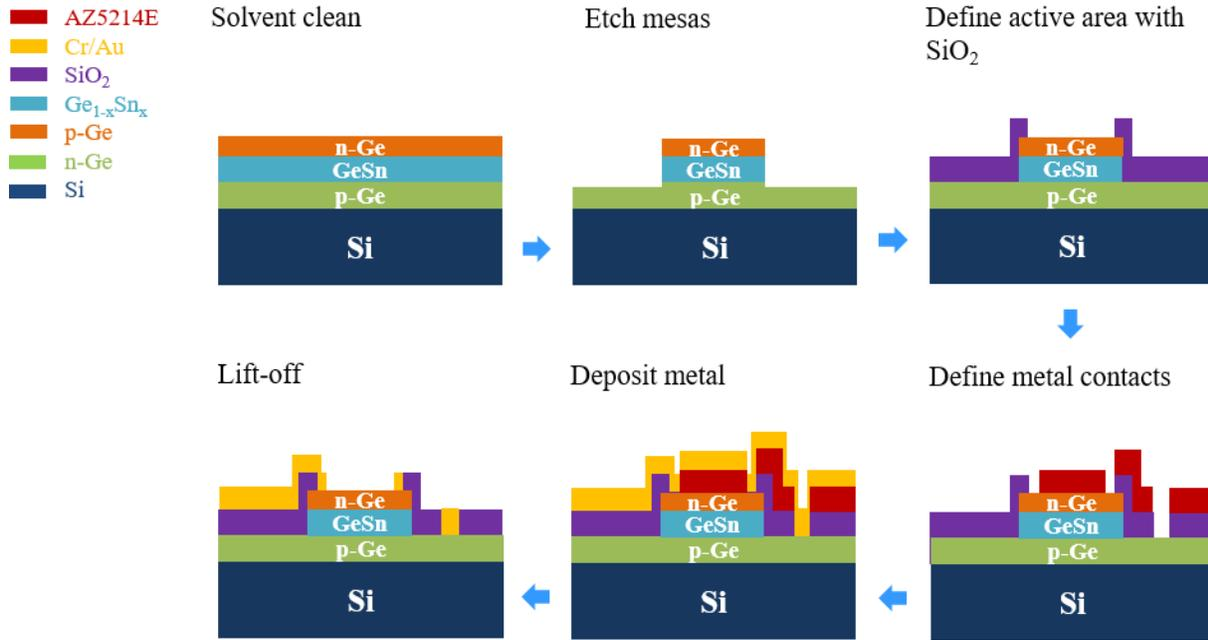
Figure 25: Fabrication process flow of first generation DHS GeSn photodiode with an absorption layer of 250 nm and with SiO<sub>2</sub> as dielectric layer
