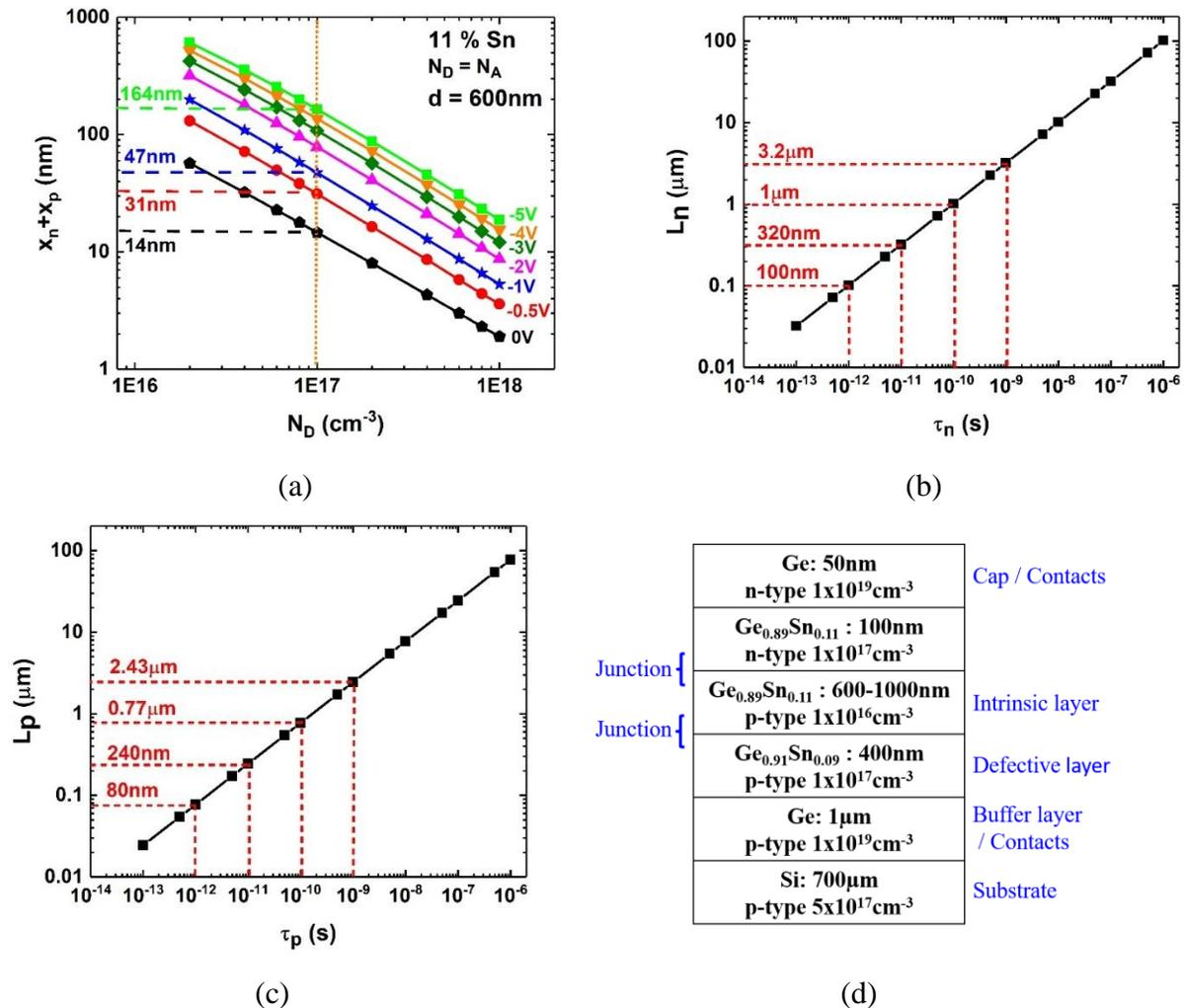
Figure 33: (a) Depletion width vs. Doping concentration of 11 % Sn assuming an intrinsic layer of 600 nm and  $N_D=N_A$ . (b) Diffusion length vs. Electron lifetime. (c) Diffusion length vs. Hole lifetime. (d) Newly proposed structure of photodiode with 11 % Sn (nominal)
