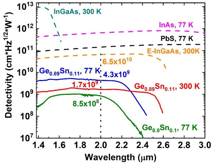
Figure 40: Spectral  $D^*$  of the 500  $\mu\text{m}$   $\text{Ge}_{0.89}\text{Sn}_{0.11}$  photodiode measured with a voltage bias of -0.1 V at 77 K (red) and 300 K (black). For comparison, the  $D^*$  spectra of several commercial detectors and our previously reported detector at 77 K (green) are also plotted. The numbers indicate the values of  $D^*$  at 2.0  $\mu\text{m}$ .
