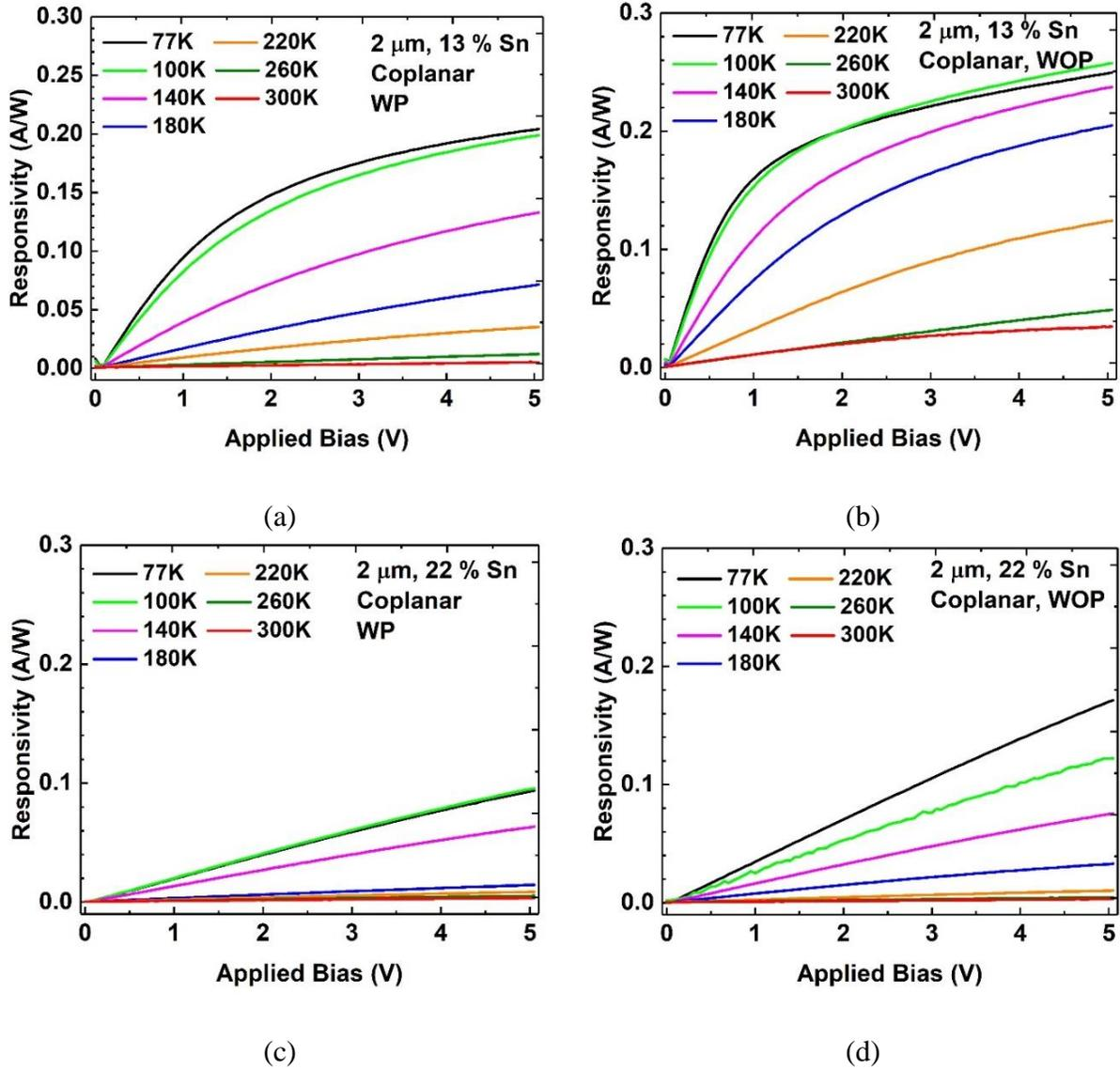
Figure 51: Temperature dependent responsivity measure at 2.0  $\mu\text{m}$  of (a) 13 % photoconductor with passivation, (b) 13 % Sn photoconductor without passivation, (c) 22 % Sn photoconductor with passivation and (d) without passivation.
