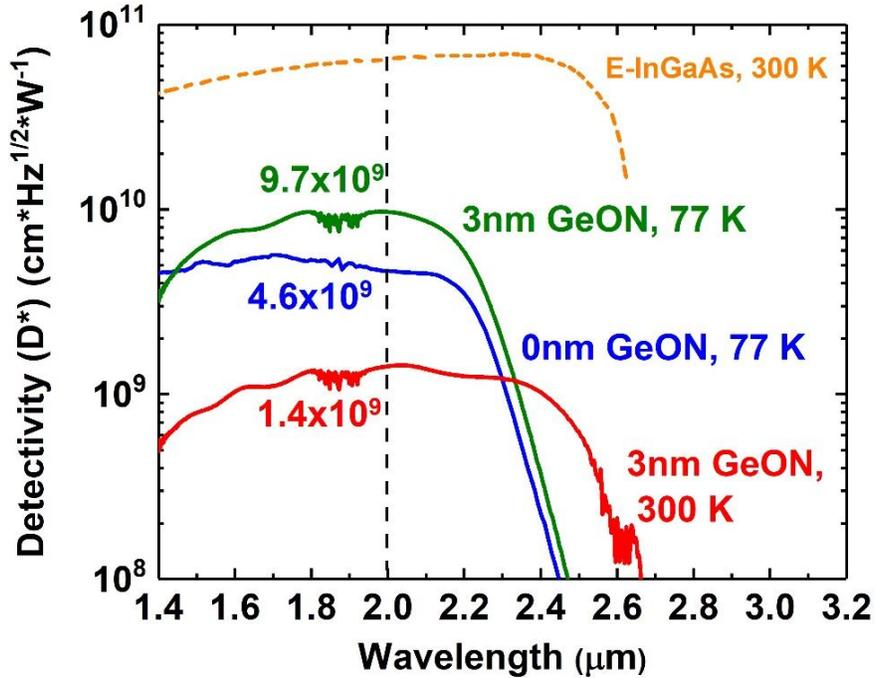
Figure 45: Spectral  $D^*$  of the  $250 \mu\text{m}$   $\text{Ge}_{0.89}\text{Sn}_{0.11}$  photodiode with 3 nm of GeON passivation measured with a voltage bias of  $-0.1 \text{ V}$  at 77 K (green) and 300 K (red). For comparison, the  $D^*$  spectra of commercial detector Ext-InGaAs and  $250 \mu\text{m}$   $\text{Ge}_{0.89}\text{Sn}_{0.11}$  at 77 K without passivation (blue) are also plotted. The numbers indicate the values of  $D^*$  at  $2.0 \mu\text{m}$ .
