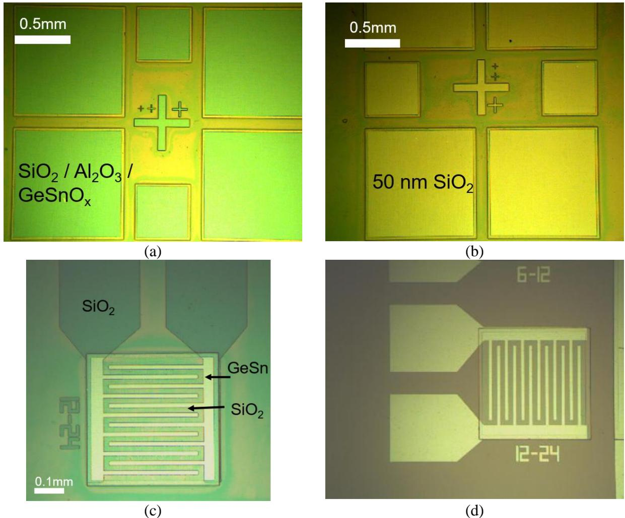
Figure 47: Top view microscope image of the photoconductor surface (a) after depositing  $\text{SiO}_2$  on passivation layer (step 3), (b) after 1<sup>st</sup>  $\text{SiO}_2$  opening step (step 4) with only 50 nm of  $\text{SiO}_2$ , (c) after 2<sup>nd</sup>  $\text{SiO}_2$  opening step (step 6), and (d) after lift-off (step 8).
