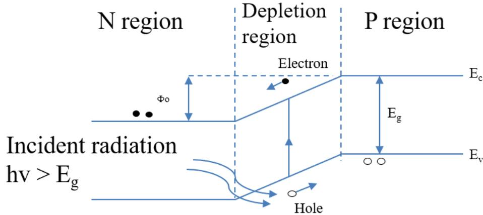
Figure 4: Band diagram p-n junction of a photodiode
