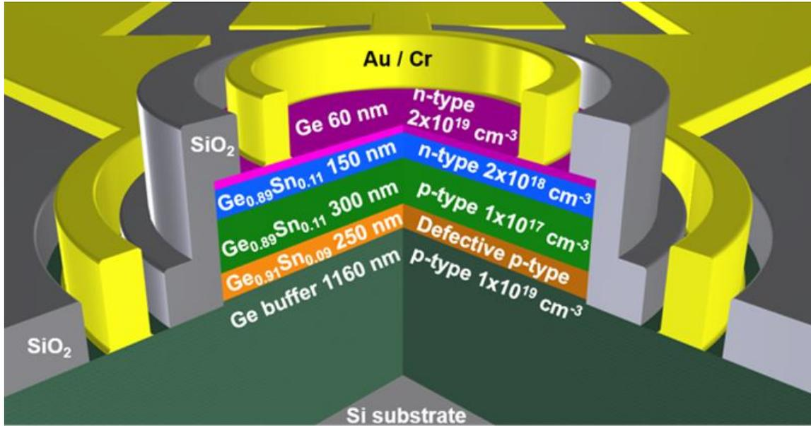
Figure 36: Schematic diagram of the  $\text{Ge}_{0.89}\text{Sn}_{0.11}$  photodiode
