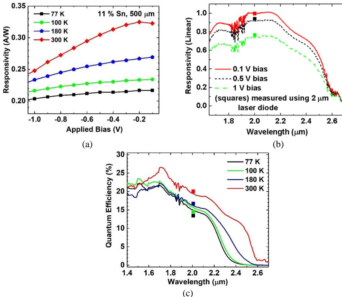
Figure 39: (a) Temperature dependent responsivity versus bias voltage measured at 2  $\mu\text{m}$  of 11 % Sn photodiode with 500  $\mu\text{m}$  in diameter. (b) Measured responsivity as a function of wavelength for different applied voltages to demonstrate the Franz-Keldysh effect. (c) Temperature-dependent spectral EQE. The dots are measured data using 2  $\mu\text{m}$  laser diode.
