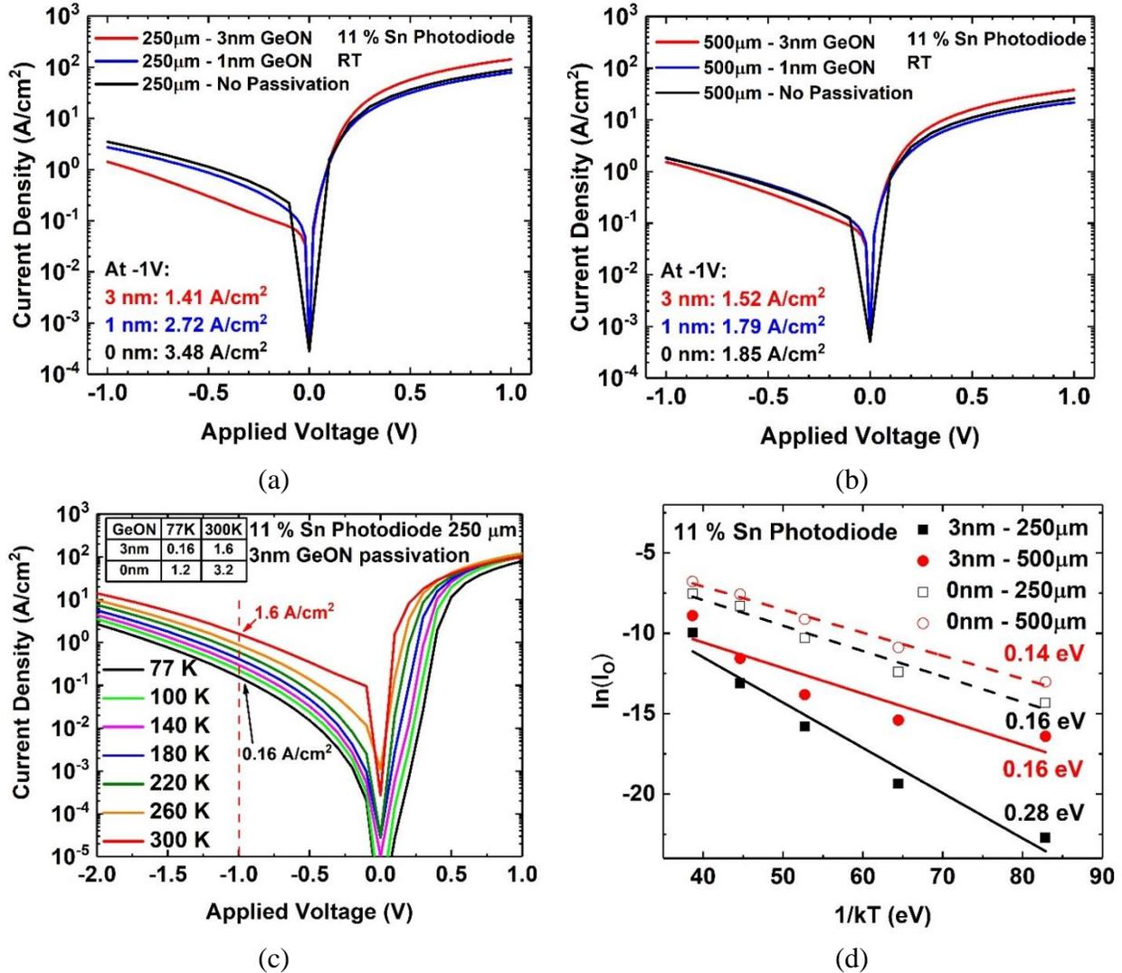
Figure 42: Room temperature current density versus voltage of 11 % Sn photodiodes with (a) 250 and (b) 500  $\mu m$  in diameter and 3nm, 1 nm, and 0 nm GeON passivation. (c) Temperature dependent current density versus voltage of 11 % Sn photodiodes with 250  $\mu m$  in diameter and 3nm GeON passivation. (d) Reverse saturation current Arrhenius plot of 11 % Sn photodiodes with 250 and 500  $\mu m$  in diameter with (solid) and without (dash) GeON passivation.
