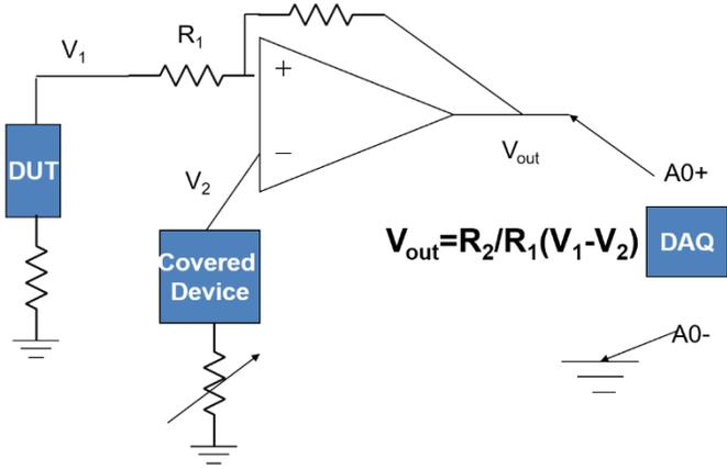
Figure 60: Circuit connection of photoconductor linear array.
