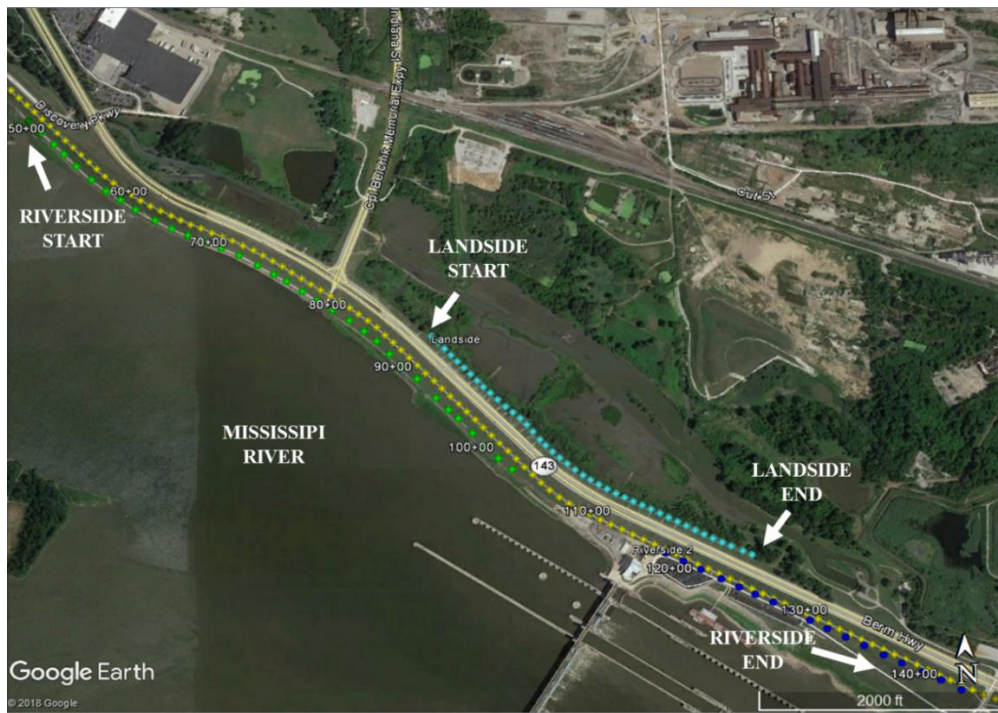
Figure 3-11. Mel Price Levee showing the start and end positions of the data acquisition process along the landside and riverside of the levee conducted using the OhmMapper.
