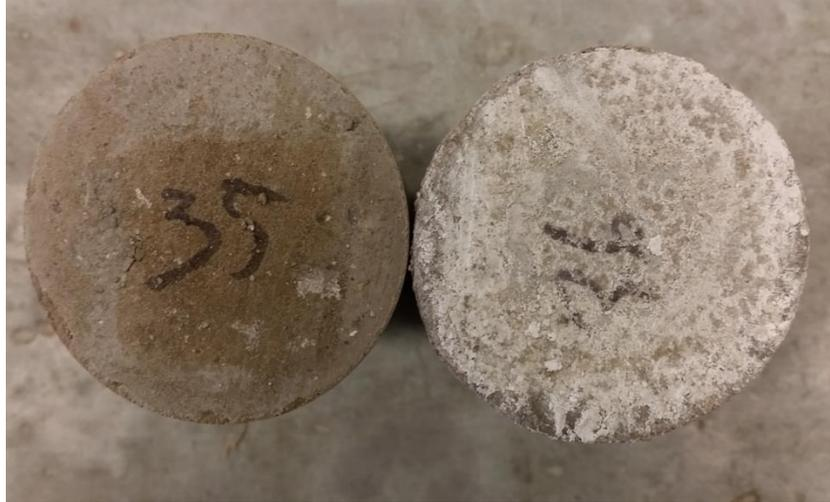
**Figure 6.** Chemical efflorescence
