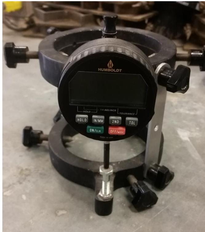
**Figure 3.** Modulus of elasticity testing collar
