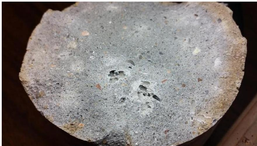
**Figure 7.** Undissolved chemicals in the mortar
