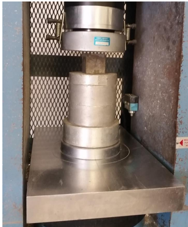
Figure 2. Compressive strength testing
