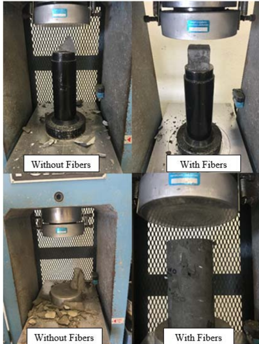
Figure 2-11. Failure of cubes and cylinders with and without steel fibers
