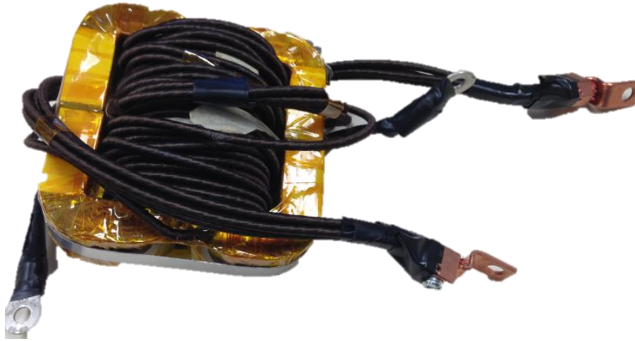
Figure 4.6. The developed 25 kHz, 5 kVA, 440 V/110 V amorphous transformer.
