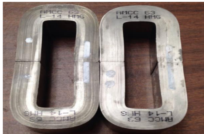
Figure 4.5. Metglas Amorphous AMCC – 63 laminated core.
