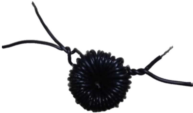
Figure 4.14. The fabricated 100 kHz nanocrystalline toroid transformer.
