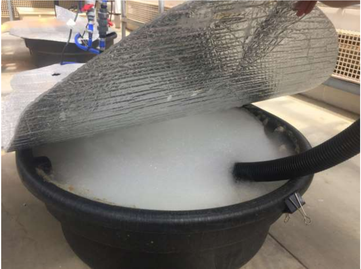
Fig. 3. Example photo of saponin foaming in NFT system ( 100 \mu\text{g}\cdot\text{mL}^{-1} ).
