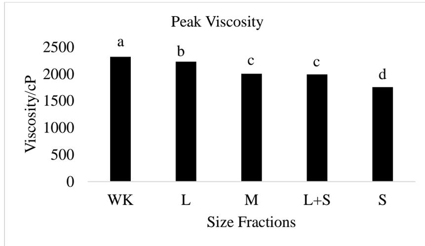
**Figure 11.** A plot of the least square mean of peak viscosity against size fractions for all 6 laboratory generated samples. WK-whole kernels, L- large brokens, M-medium brokens, L+S- a 1:1 mixture of large and small brokens, S-small brokens. Values followed by the same letter are not significantly different ( $P > 0.05$ ).
