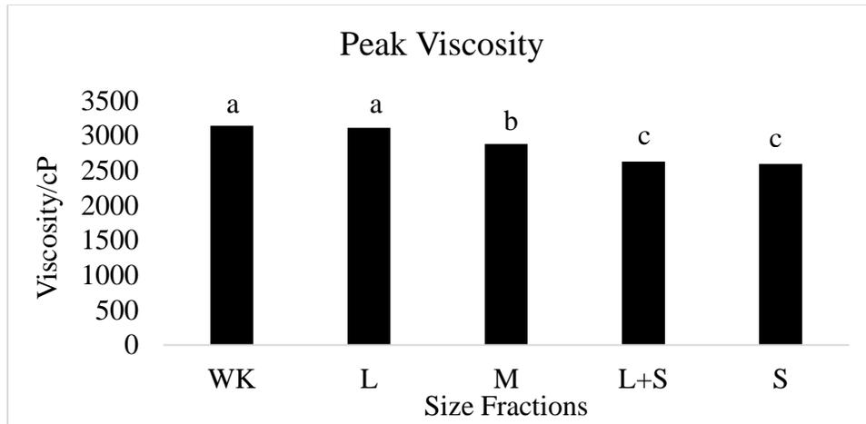
**Figure 2.** Peak viscosity of size fractionated conventional industrial rice (non-parboiling stream). WK-whole kernels, L- large broken, M-medium broken, L+S- a 1:1 mixture of large and small broken, S-small broken.
