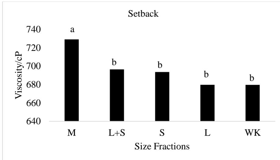
**Figure 13.** A plot of the least square mean of setback viscosity against size fractions for all 6 laboratory generated samples. WK-whole kernels, L- large broken, M-medium broken, L+S- a 1:1 mixture of large and small broken, S-small broken.
